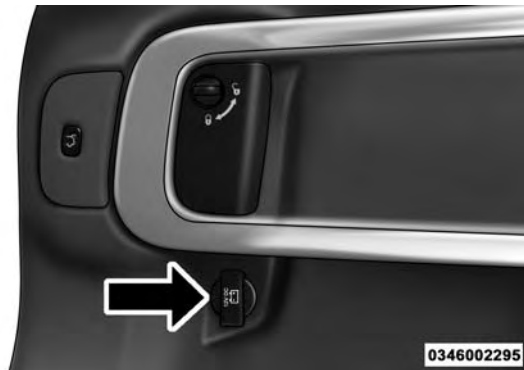
Rear Power Outlet
