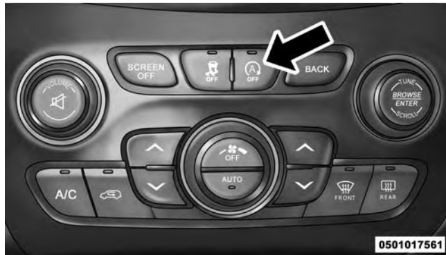
STOP/START OFF Switch
