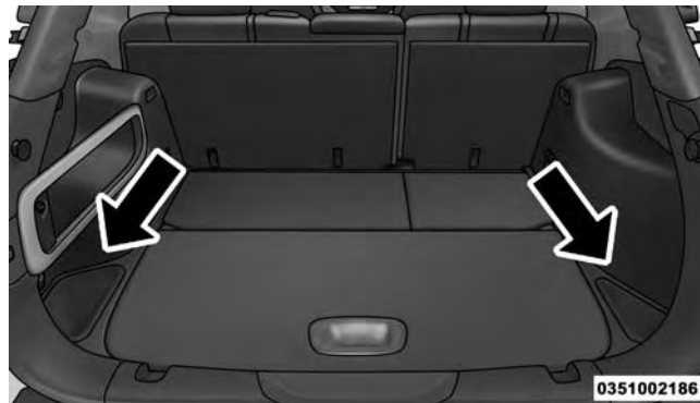
Rear Storage Bins
