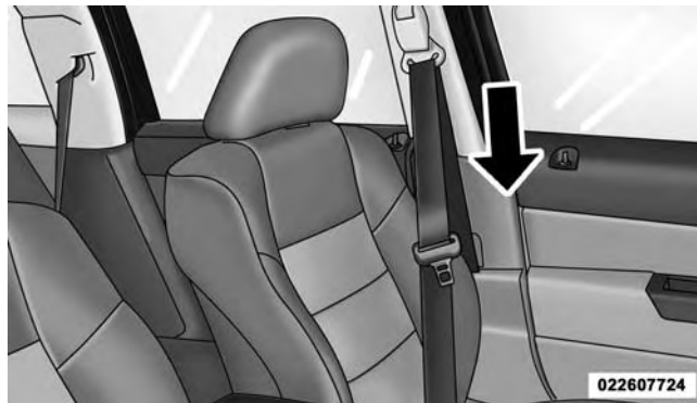
Pulling Out The Latch Plate
