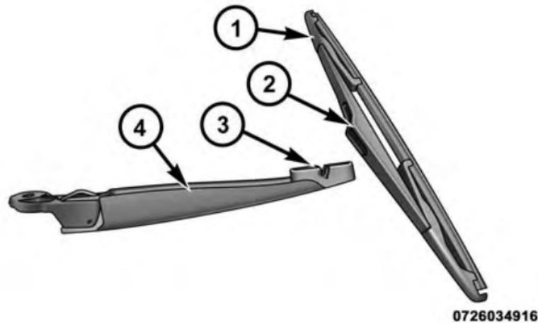
Wiper Blade Removed From Wiper Arm
