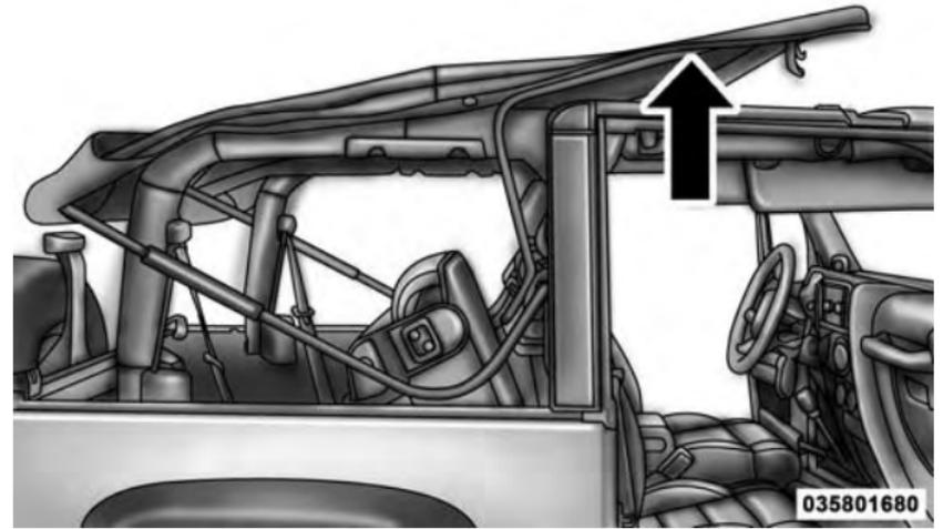
18. Tuck the fabric and the check straps between the bows and as far inward as possible. This will keep any portion of the top from flapping outside of the vehicle.
