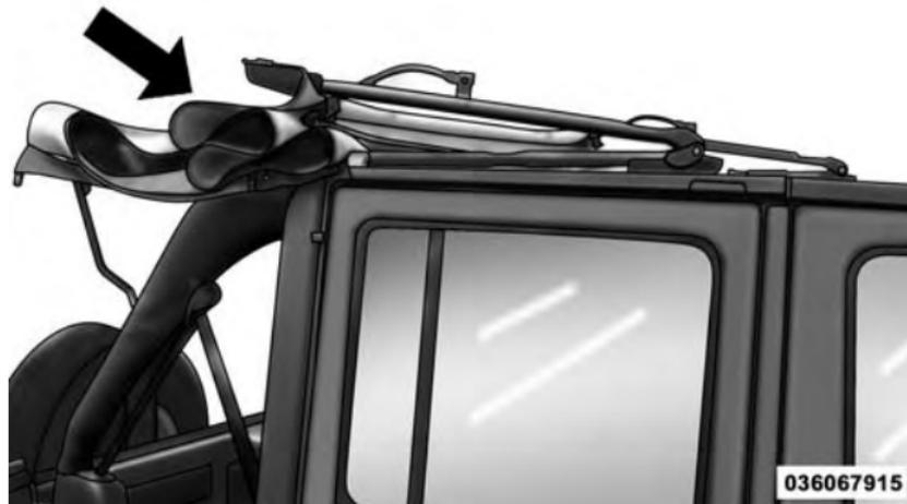
17. Release the side bows by pushing down on the latch above the front of the rear door. Push the top rearward to disengage. Repeat this step on the other side.
