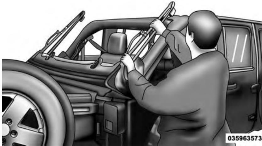
20. Tuck the fabric and the check straps between the bows as far inside as possible. This will keep any portion of the top from flapping outside of the vehicle.
