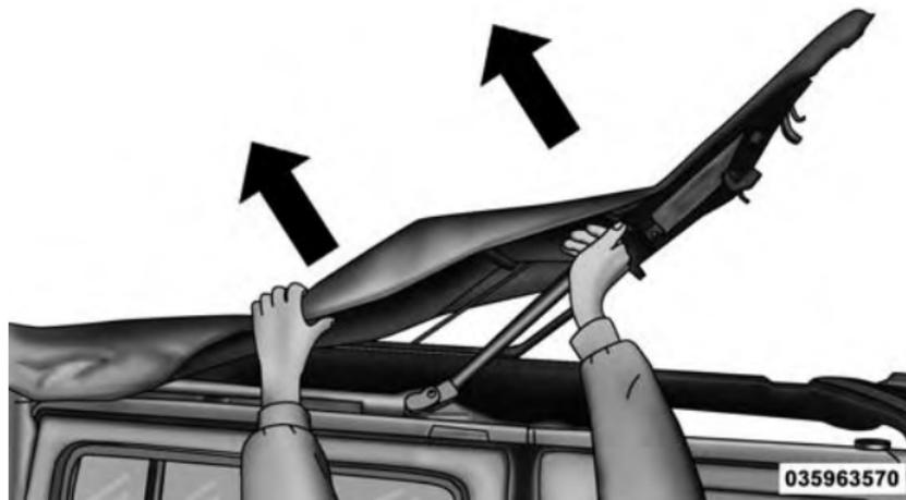
15. Fold back the front section of the top, pulling the fabric rearward. Gently rest the header on top of the rear portion of the deck.
