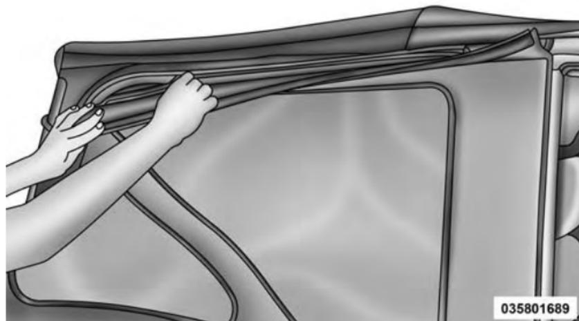
13. Locate the black swing gate bar. Slide the swing gate bar over the receiver at the bottom inside of the rear window. The spongy part of the seal should be down and pointed outward to seal with the swing gate when closed.
