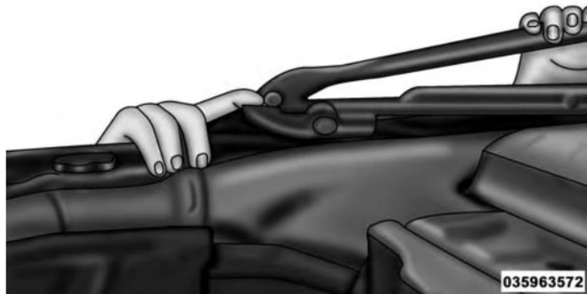
18. Before lowering the top, open the swing gate to prevent possible damage to the rear center high-mounted brake light. Grasp the folded side bows and
