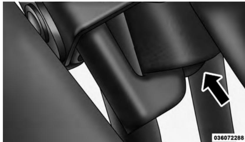
5. The tether strap **must** be hooked onto the pivot bracket prior to removal of soft top from vehicle (both sides).
