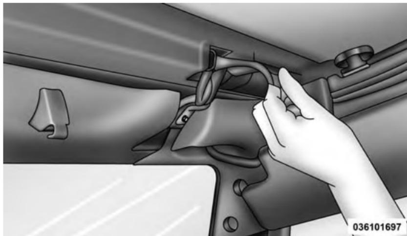
3. Make sure to slide the plastic sleeves forward to unlock the Sunrider links.
