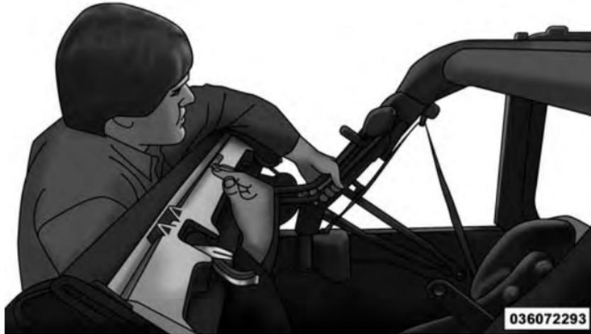
5. Lower the pivot bracket onto the sport bar bracket mounting tab in a downward motion to lock into tab.
