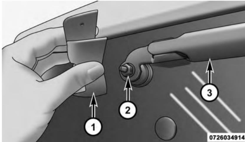
Wiper Arm With Pivot Cap Removed
