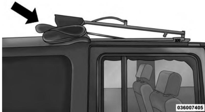
7. Secure the top by using the two provided straps. Each strap will wrap around the side bow and Velcro to itself; use one strap on each side of the vehicle.
