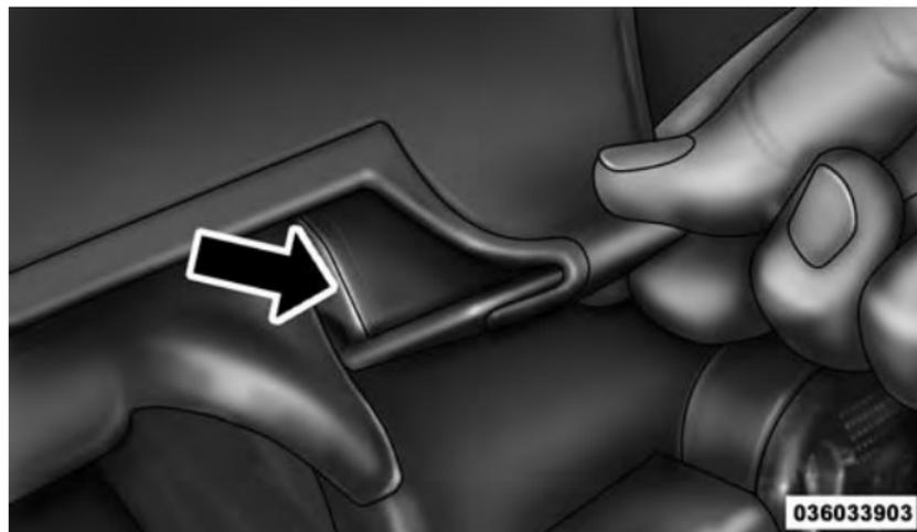
20. Complete the installation of the sail panel by inserting the rest of the retainer into the body channel.
