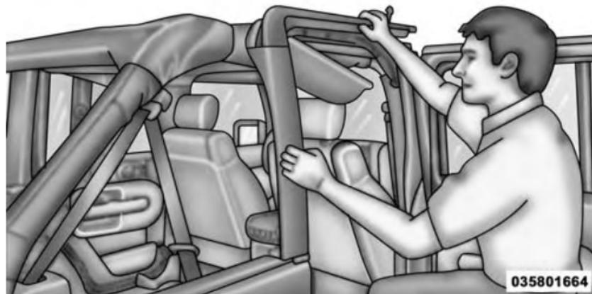
3. Position the top of the door frame against the metal sport bar and push onto the side bar making sure not to pinch the material of the sports bar covers and to ensure it is properly positioned on the seal above the front of the rear door.
