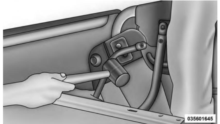
5. Unzip the zipper on the sport bar cover to expose the pivot brackets. Remove the brackets using a #T30 Torx head driver. Recover and re-zip the sports bar cover. Store the pivot brackets and screws in a safe place.
