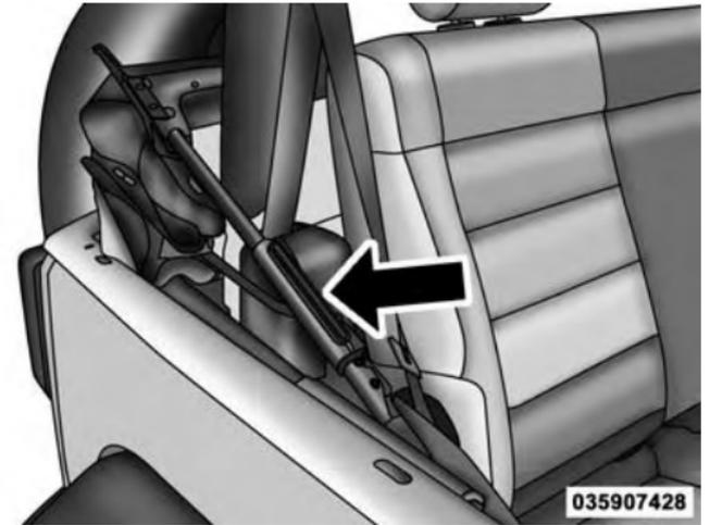
4. Standing on the side of the vehicle, lift the top by the side bow and the 2-bow (middle bow) up and over the sports bar until the header rests on the top of the windshield frame.
