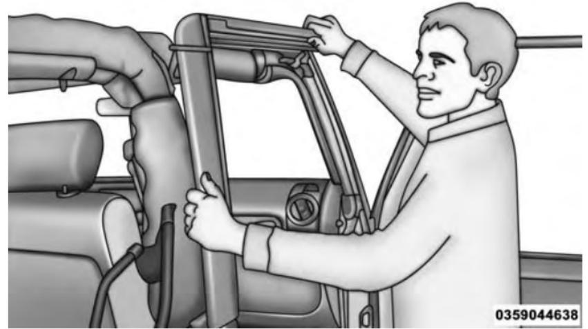
3. After the door frame pin has been set into the body side hole, carefully set the front of the door frame into the rubber seal at the top of the windshield.
