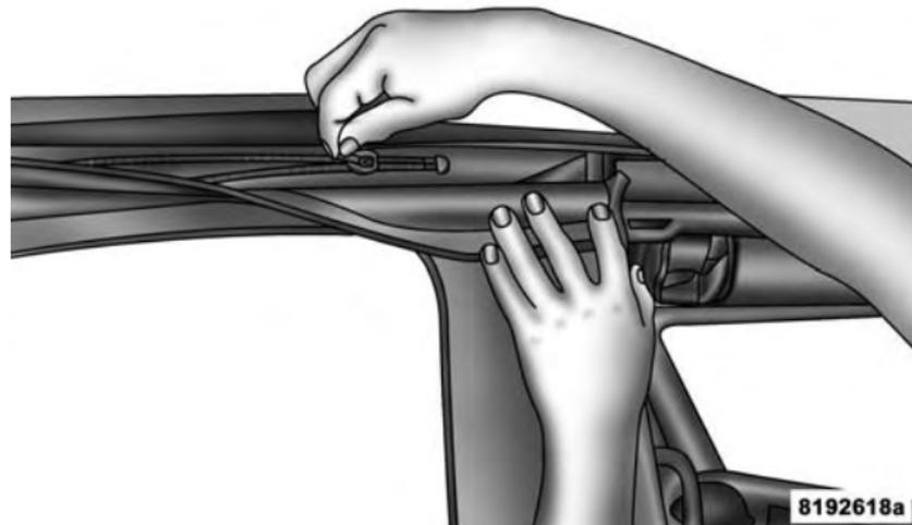
13. Insert the front retainer of the window into the door channel, making sure the retainer is fully seated and properly positioned on the door frame. Failure to do so can result in wind and water leaks or damage to the window.
