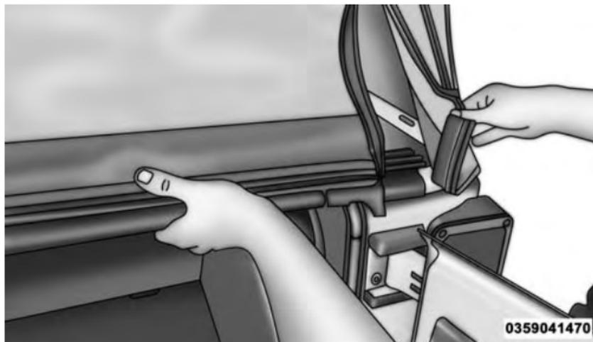
19. Insert the rear window retainer into the swing gate bracket on both the left and right sides.
