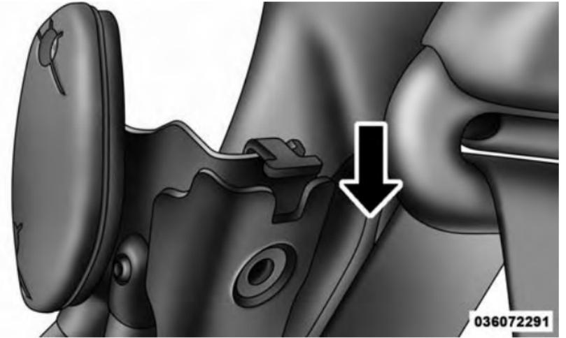
6. Install the pivot bracket bolts back into place using a 10.0 mm wrench or socket driver. Secure them until they are snug, being careful not to cross-thread the screws or overtighten.
