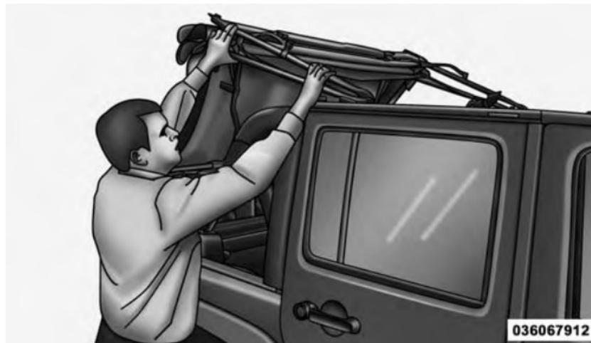
19. Gently slide the side bows off the door frame track and lower the top down into the vehicle.
