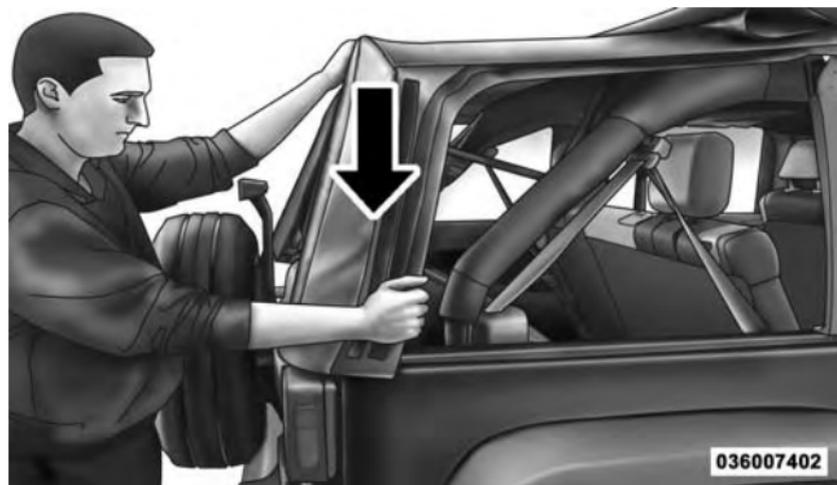
3. Rotate the header forward.
