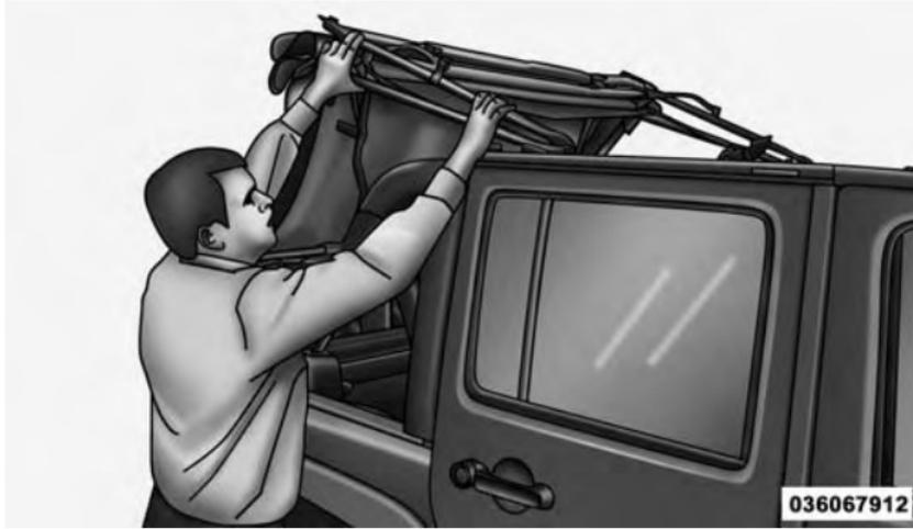
6. Ensure that the top locks into the Sunrider locking mechanisms that are located above the front of the rear doors.
