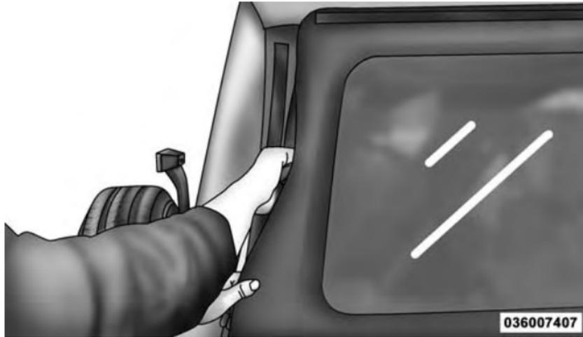
7. To install the side windows, affix the window temporarily by attaching to the Velcro in the rear corner. Start the zipper but close only about 1 in (2.5 cm).
