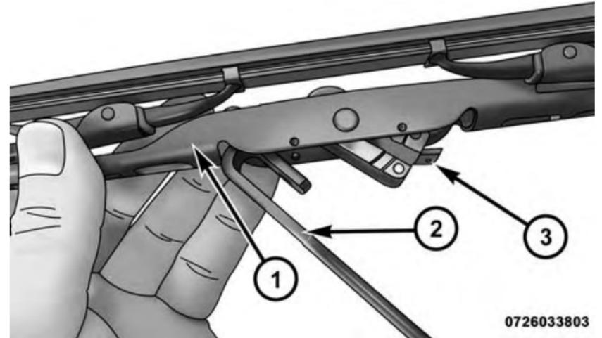
**Wiper Blade Removed From Wiper Arm**
