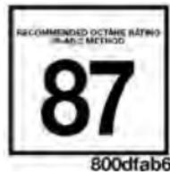
This engine is designed to meet all emissions regulations and provide optimum fuel economy and performance when using high quality unleaded "Regular" gasoline having a posted octane number of 87 as specified by the (R+M)/2 method. The use of higher octane "Premium" gasoline is not required, as it will not provide any benefit over "Regular" gasoline in these engines.
