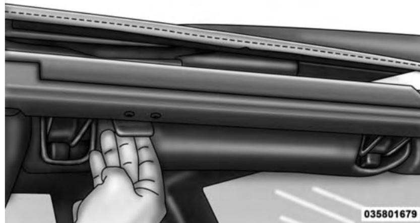
17. Before lowering the top, open the swing gate to prevent possible damage to the rear center high-mounted brake light. Move to the front of the vehicle. Grasp the side bow behind the header and lift the top, folding it toward the rear of the vehicle.
