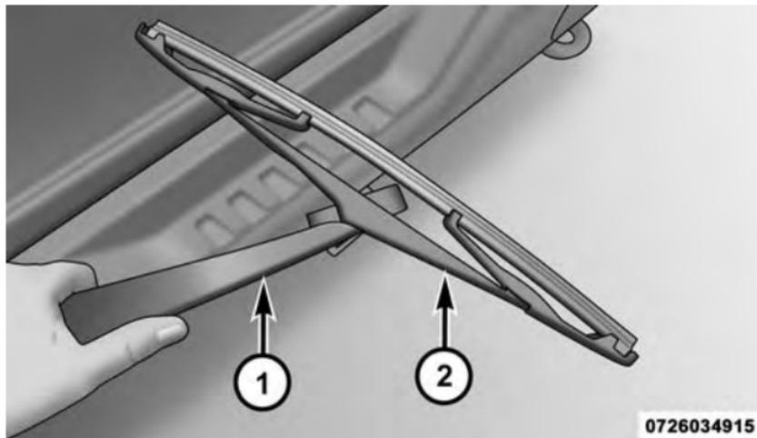
Wiper Blade Removed From Wiper Arm
