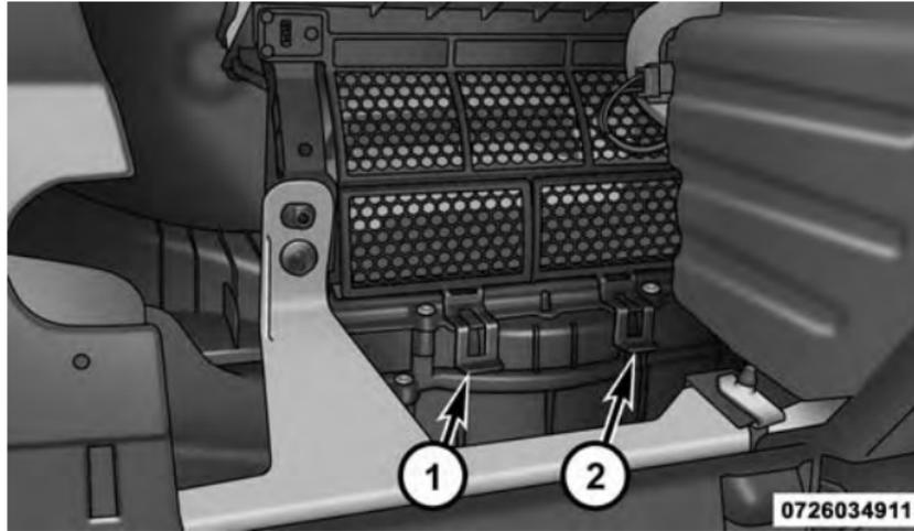
**Air Filter Retaining Tabs**
