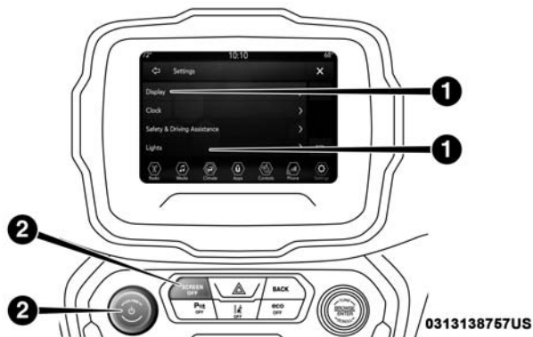
Uconnect 4 With 7-inch Display Buttons On The Touchscreen And Buttons On The Faceplate
