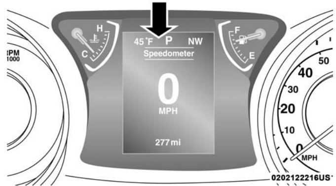
3.5 Inch Instrument Cluster Display Location
