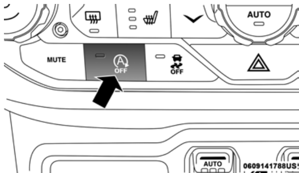
STOP/START Off Switch
