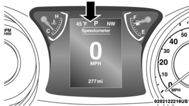
3.5 Inch Instrument Cluster Display Location
