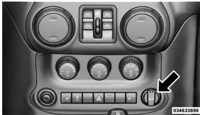
Front Power Outlet
