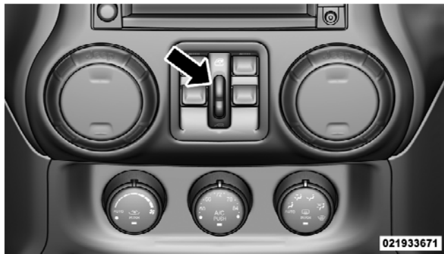
Window Lockout Switch
