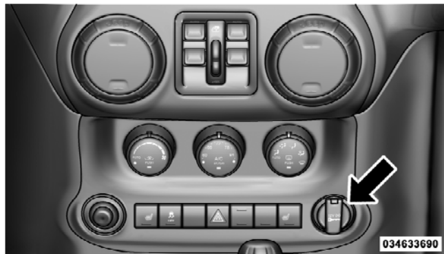
Front Power Outlet
