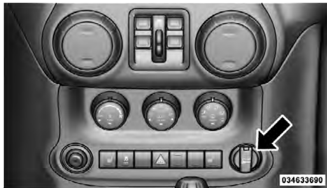
Front Power Outlet
