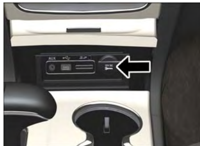
Front Power Outlet
