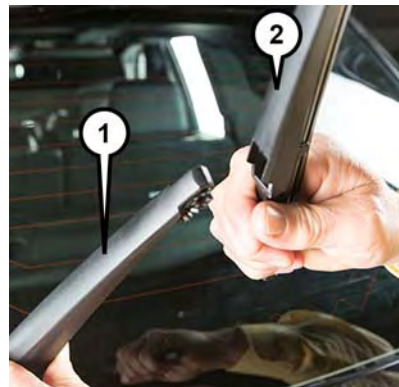
Wiper Blade Removed From Wiper Arm
