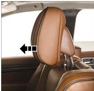
Active Head Restraint (Tilted)
