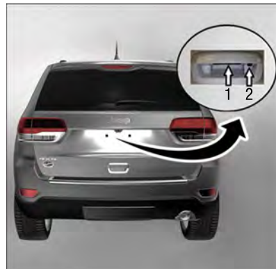
Electronic Liftgate Release/Liftgate Passive Entry Location
