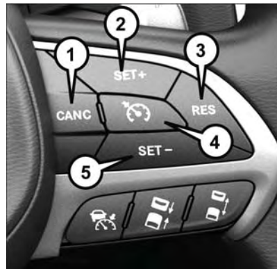
Electronic Speed Control Switches
