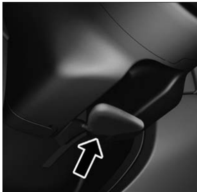
Manual Tilt/Telescoping Steering Column Handle
