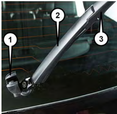
Wiper Blade In Folded Out Position
