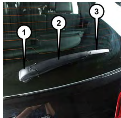
Wiper Pivot Cap In Unlocked Position
