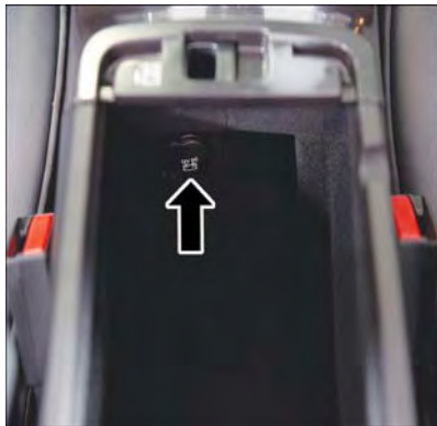
Center Console Power Outlet
