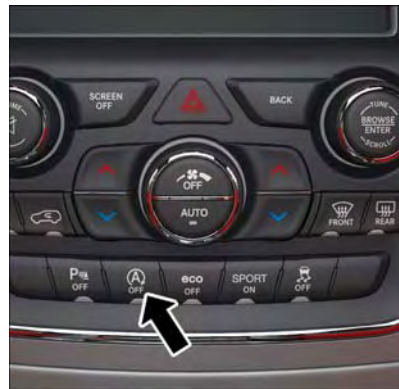
STOP/START Off Switch
