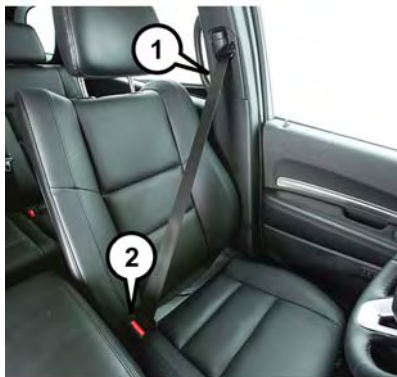
Pulling Out The Latch Plate
