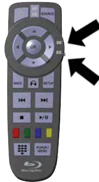
RSE System Remote Control Channel Selectors
