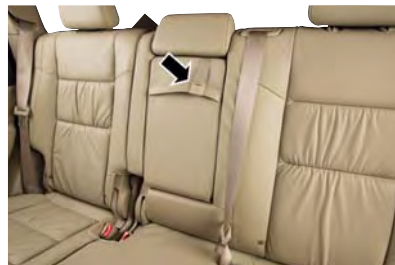
Center Seat Position Arm Rest Tether Attached
