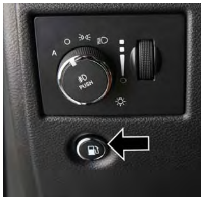
Fuel Filler Door Release Switch
