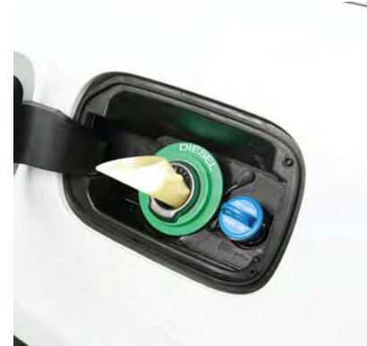
Emergency Fuel Fill Location
