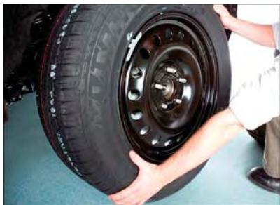
Installing Spare Wheel/Tire
