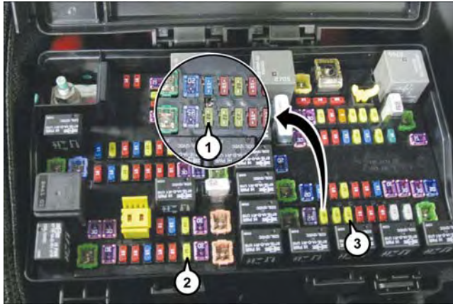
Power Outlet Fuse Locations
