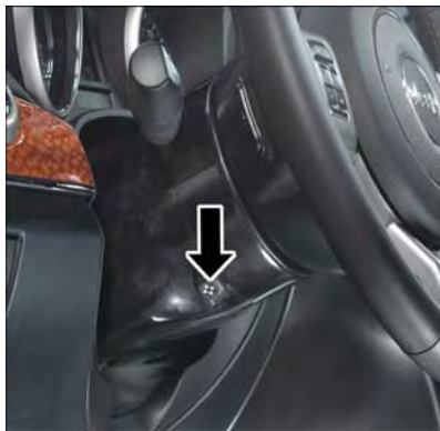
Power Tilt/Telescoping Control
