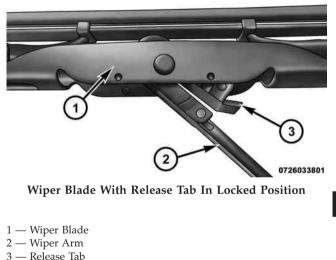
2. To disengage the wiper blade from the wiper arm, press the release tab on the wiper blade and while holding the wiper arm with one hand, slide the wiper blade down towards the base of the wiper arm.
