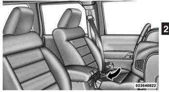
**Inserting Latch Plate Into Buckle**
