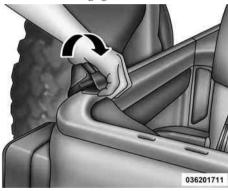
13. The swing gate brackets do not need to be removed unless the hard top is being installed. To remove the the top.14. Grasp the front side bow behind the header, and lift the top.
