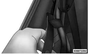
5. The tether strap **must** be hooked onto the pivot bracket prior to removal of soft top from vehicle (both sides).
