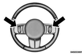
Remote Sound System Controls (Back View Of Steering Wheel) The right-hand control is a rocker-type switch with a push-button in the center and controls the volume and mode of the sound system. Pushing the top of the rocker switch will increase the volume, and pushing the bottom of the rocker switch will decrease the volume.
