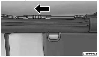
6. As you begin to lower the top, fold the sail panels so 7. Release the Sunrider® latch (both sides). that they rest on top of the soft top.
