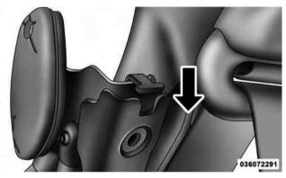
6. Install the pivot bracket bolts back into place using a 10.0 mm wrench or socket driver. Secure them until they are snug, being careful not to cross-thread the screws or overtighten.
