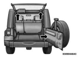
6. Locate the wire harness on the left rear inside corner of the vehicle.
