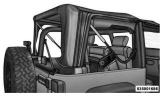
9. Partially install the sail panel retainers into the body side channel, leaving the last 3 in (7.6 cm) toward the rear window loose (on both sides). Pulling down on the rear roof bow (3–bow) will aid to reach the channel with the retainers.
