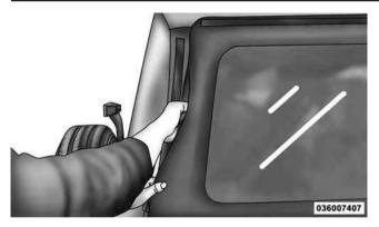
15. Locate the black swing gate bar. Slide the swing gate bar over the receiver at the bottom inside of the rear window. The spongy part of the seal should be down and pointed outward to seal with the swing gate when closed.
