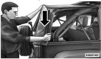
3. Rotate the header forward.
