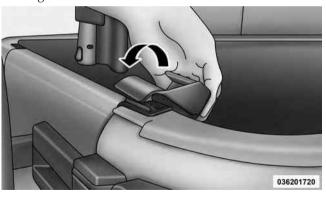
11. Ensure that the straps are positioned correctly before pulling the sail panels over the rear roof bow (4–bow).
