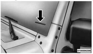
Vehicle Identification Number NOTE: It is illegal to remove or alter the VIN plate.
