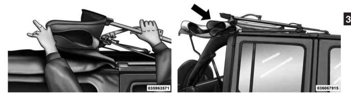
17. Release the side bows by pressing down on the latch above the front of the rear door. Push the top rearward to disengage. Repeat this step on the other side.
