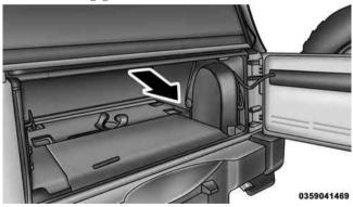
top and down to the left lower corner. **Zipper pulls** will stay on the rear window. Pull down on the rear window to disengage it from the zipper on the top cover.
