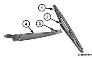
Wiper Blade Removed From Wiper Arm
