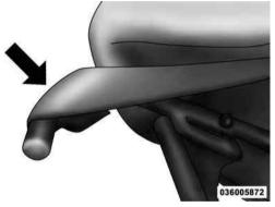
Partially install the sail panel retainers into the body side channel, leaving the last 3 in (7.6 cm) toward the rear window loose (on both sides). Pulling down on the rear roof bow (4–bow) will aid in reaching the channel with the retainers.
