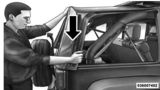
12. To install the side windows, affix the window temporarily by attaching it to the Velcro® in the upper rear corner. Start the zipper but close only about 1 in (2.5 cm).
