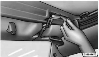
4. Release the sail panel retainers from the body side 5. Fold the sail panels so that they rest on top of the soft top.
