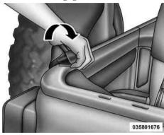
14. Completely release the latches from the loops on the windshield frame. If your vehicle is not equipped with the Sunrider® package, proceed to Step 15.
