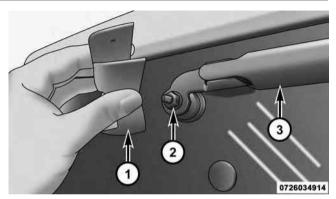
Wiper Arm With Pivot Cap Removed
