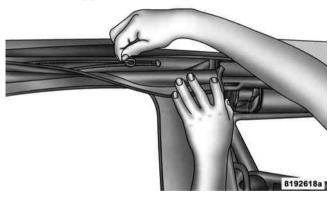
8. Insert the front retainer of the window into the door channel, making sure the retainer is fully seated and
