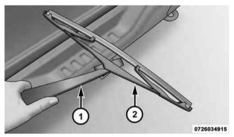
Wiper Blade Removed From Wiper Arm
