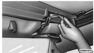
4. Release the sail panel retainers from the body side channel at the rear corners of the vehicle.
