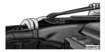
18. Before lowering the top, open the swing gate to prevent possible damage to the rear center highmounted brake light. Grasp the folded side bows and slide the top along the door frame track to the rear door frame.
