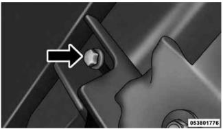
**Underside Bolt** 3. Remove the side step assembly.
