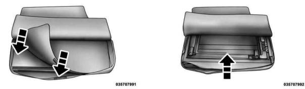
Insert the left-side Freedom panel into the bag with the Unfold the outer flap and zip the Freedom bag closed. latches facing upward.
