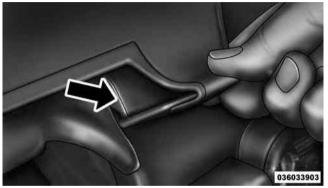
20. Complete the installation of the sail panel by inserting the rest of the retainer into the body channel. 21. Close the header latches and return the sun visors to their secured position.
