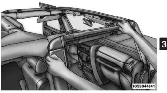
4. Screw the knobs back into the door frame and fold for storage. Store in a secure location.
