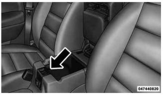
Center Console USB/AUX Connector Port Once the audio device is connected and synchronized to the vehicles iPod®/USB/MP3 control system (iPod® or
