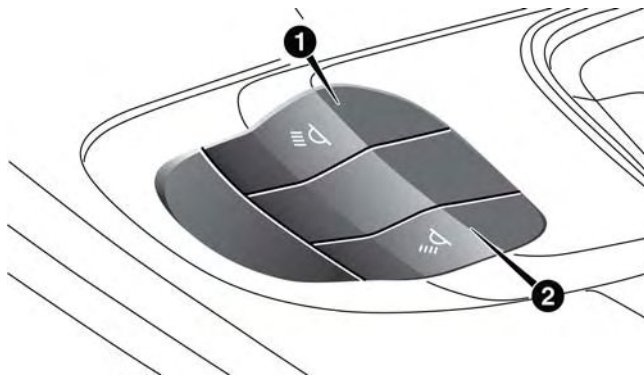
Courtesy Light Switches
