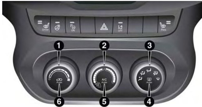
Manual Temperature Controls (MTC)
