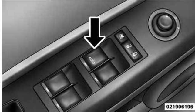
Power Window Switch Location
