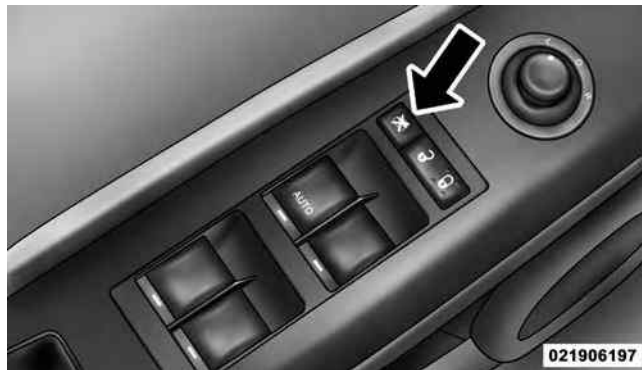
Window Lockout Switch
