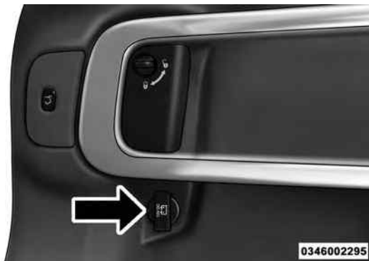
Rear Power Outlet
