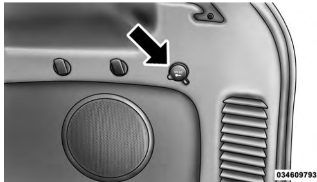
Rear Power Outlet
