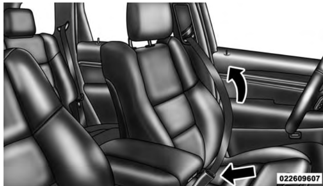
Removing Slack From Belt
