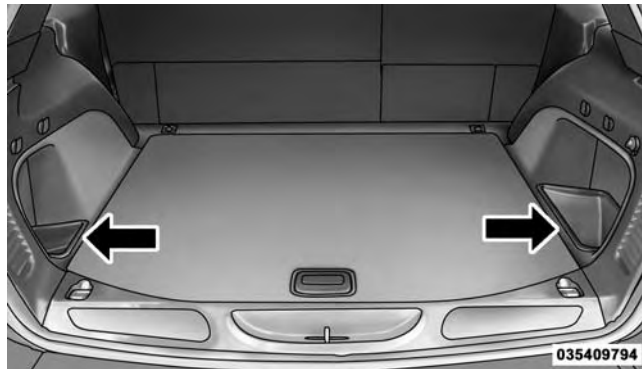
Rear Storage Bins
