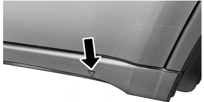
Lift Point Symbol On Sill Molding
