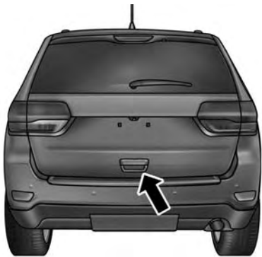
Electronic Liftgate Handle/Liftgate Passive Entry Location
