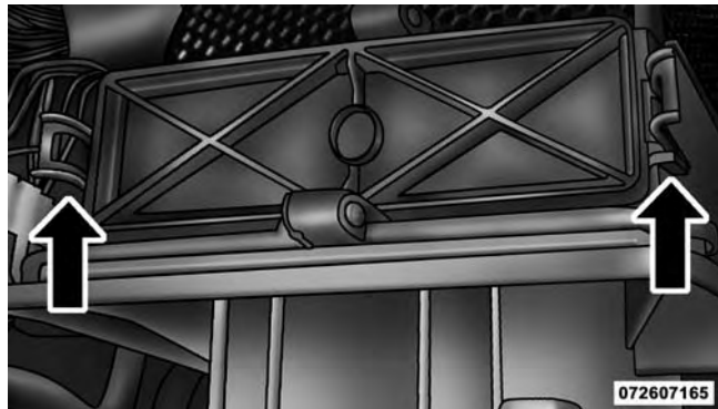
A/C Air Filter Replacement
