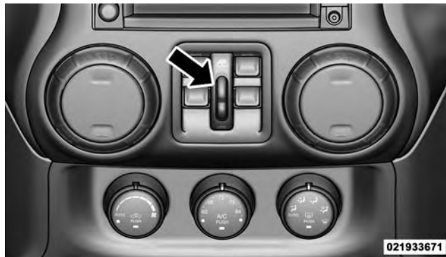
Window Lockout Switch
