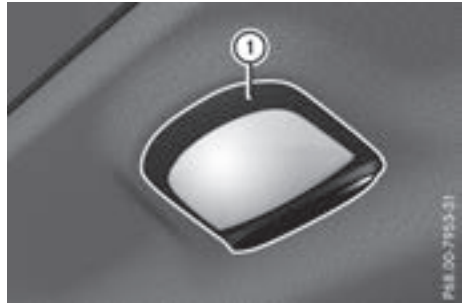
Rear overhead control panel (third row of seats)
