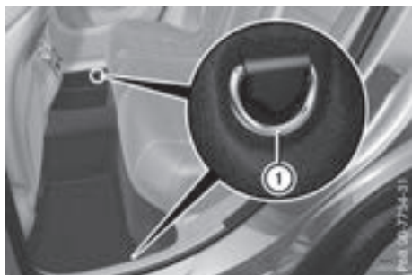
① Cargo tie-down rings in the rear-compartment footwell (vehicles with cargo net)
