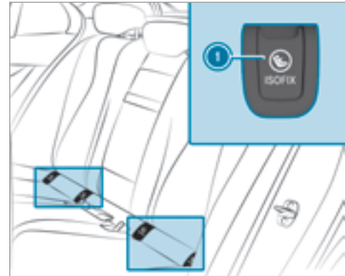
① LATCH-type (ISOFIX) mounting brackets
