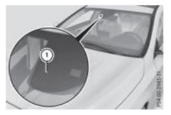
Lane Keeping Assist monitors the area in front of your vehicle by means of multifunction camera (1) which is attached behind the top of the windshield. Lane Keeping Assist detects lane markings on the road and can warn you before you leave your lane unintentionally.
