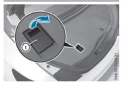
Under the trunk floor you can find a bracket for TIREFIT and the vehicle tool kit, etc.
