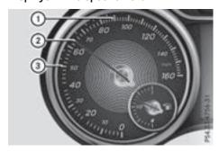
When Distance Pilot DISTRONIC PLUS is activated and there are no vehicles detected in front, one or two segments ② in the set speed range light up.
