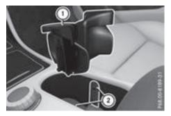
➤ To install: insert cup holder into lateral curved sections ② in the stowage compartment. Insert the cup holder so that the wedge
