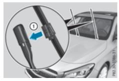
▶ Insert the new wiper blade into the wiper arm in the direction of arrow (1).
