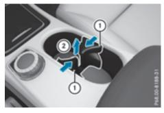
The cup holder and the rubber mat underneath can be removed for cleaning. Clean them with clean, lukewarm water only.
