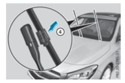
▶ Remove the wiper blade in the direction of arrow (4) away from the wiper arm.
