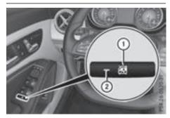
▶ To activate/deactivate: press button ①. If indicator lamp ② is lit, operation of the rear side windows is disabled. Operation is only possible using the switches in the driver's door. If indicator lamp ② is off, operation is possible using the switches in the rear compartment.
