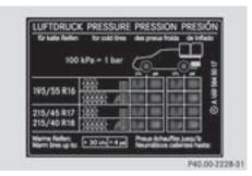
The load conditions "partially laden" and "fully laden" are defined in the table for different numbers of occupants and amounts of luggage. The actual number of seats may differ.
