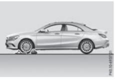
▶ Place chocks or other suitable items under the front and rear of the wheel that is diagonally opposite the wheel you wish to change.
