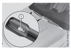
► Remove protective film ① of the service indicator on the tip of the wiper blade.
