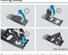
If your vehicle is equipped with a wheel chock, it can be found in the tire-change tool kit (> page 270).
