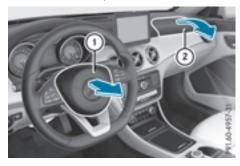
Driver's air bag (1) deploys in front of the steering wheel. Front-passenger front air bag (2) deploys in front of and above the glove box.
