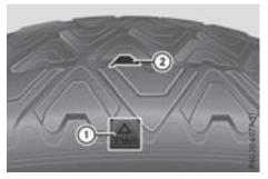
Marking (1) shows where bar indicator (2) for tread wear is integrated into the tire tread. Treadwear indicators (TWI) are required by law. Six indicators are positioned on the tire tread. They are visible once a tread depth of approximately 1/16 in (1.6 mm) has been reached. If this is the case, the tire is so worn that it must be replaced.
