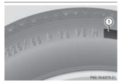
In addition to the load-bearing index, load index ① may be imprinted after the letters that identify speed rating on the sidewall of the tire. Speed rating (> page 302).
