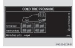
The tire pressure table contains the recommended pressures for cold tires for various operating conditions, i.e. differing load and speed conditions.
