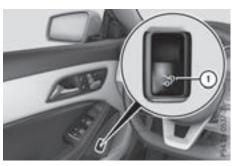
▶ **To open:** pull remote operating switch ① for the trunk lid until the trunk lid opens.
