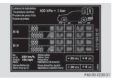
Some tire pressure tables show only the rim diameters instead of the full tire size, e.g. **R18**. Rim diameter is part of the tire size and can be found on the tire sidewall (▷ page 302).
