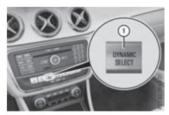
Press DYNAMIC SELECT button ① as many times as necessary until the desired drive program is selected.
