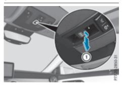
Reset the panorama roof with power tilt/sliding panel or the roller sunblind if the panorama roof with power tilt/sliding panel or the roller sunblind does not move smoothly.
