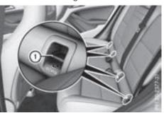
▶ Install the LATCH-type (ISOFIX) child restraint system on both LATCH-type (ISOFIX) securing rings (1).
