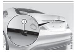
Rear view camera ① is an optical parking and maneuvering aid. It shows the area behind your vehicle with guide lines in the multimedia system display.
