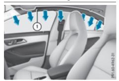
Window curtain air bags (1) are integrated into the side of the roof frame and deployed in the area from the A-pillar to the C-pillar.
