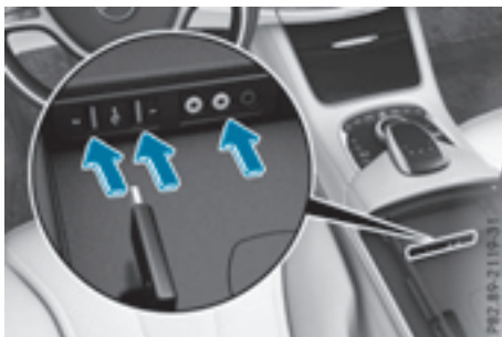
Connections in the storage compartment under the armrest in vehicles with rear climate control
