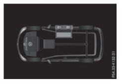
The engine and electric motor are switched off. The arrows for the energy flow are not shown. The condition of charge of the high-voltage battery is shown when the SmartKey is in position 2 in the ignition lock.
