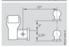
When choosing a ball coupling, the dimensions stated in the illustration must not be exceeded.
