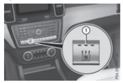
► To activate or deactivate "Immediate preentry climate control": press button ①. The blue or red indicator lamp in the button lights up or goes out.
