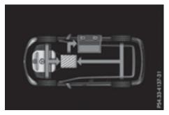
The engine powers the vehicle. The electric motor is operating as a generator, e.g. in overrun mode and when braking (▷ page 24). The
