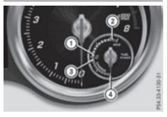
The power display for the electric motor is located on the right-hand side of the instrument cluster.
