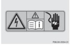
All components of the hybrid drive system are marked with yellow warning stickers that warn you of the danger of high voltage. The cables of the vehicle's high-voltage electrical system are orange in color.
