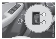
▶ Pull switch ②. Indicator lamp ① flashes and the Please Wait Depressurizing Tank message appears in the multifunction display. If the fuel filler cap is unlocked, indicator lamp ① lights up.
