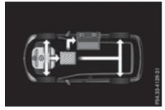
The engine powers the vehicle. The engine also powers the electric motor. The electric motor operates as a generator. The high-voltage battery is being charged.
