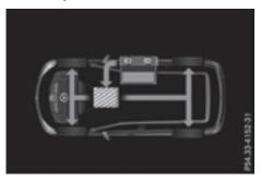
The electric motor powers the vehicle. The highvoltage battery supplies energy to the electric motor.
