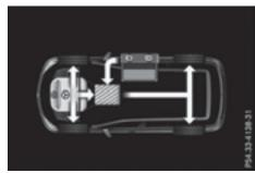
The engine powers the vehicle. If the vehicle is approaching a downhill gradient with a high potential for energy recuperation, the condition of charge of the high-voltage battery is intentionally kept low or intentionally reduced.
