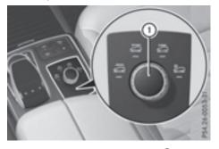
► Turn DYNAMIC SELECT controller ① as many times as necessary until the desired drive program is selected.
