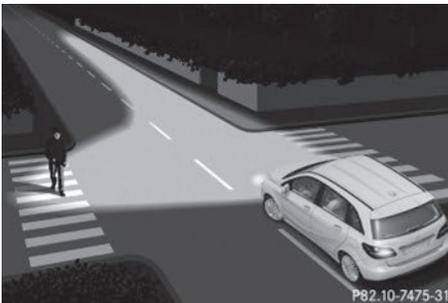
The cornering light function improves the illumination of the road over a wide angle in the
