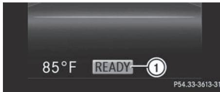
When the drive system is started and the vehicle is ready to drive, READY indicator ① appears in the multifunction display. This indicates that the vehicle is operational.
