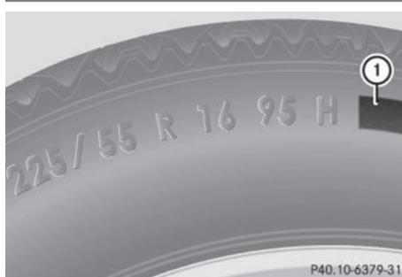
In addition to the load-bearing index, load index ① may be imprinted after the letters that identify speed rating on the sidewall of the tire. Speed rating (▷ page 270).
