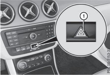
► **To switch on the hazard warning lamps:**
