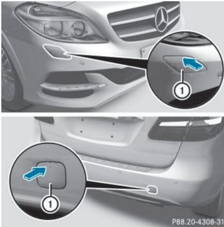
The brackets for the screw-in towing eye are located in the bumpers. They are at the rear and at the front, under covers ①.
