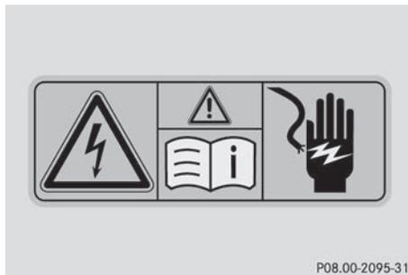
All of the vehicle's high-voltage electrical system components are marked with yellow warning stickers which warn you about high voltages. The cables of the vehicle's high-voltage electrical system are orange.
