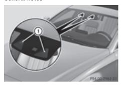
Lane Keeping Assist monitors the area in front of your vehicle with camera (1), which is mounted at the top of the windshield. Active Lane Keeping Assist detects lane markings on the road and can warn you before you leave your lane unintentionally.
