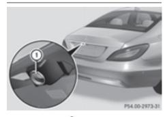
Rear view camera ① is an optical parking and maneuvering aid. It shows the area behind the vehicle with guide lines in the multimedia system.
