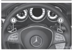
In the manual drive program, you can change gears manually using steering wheel paddle shifters (1) and (2).
