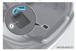
The TIREFIT kit, the vehicle tool kit, etc. are located in the stowage compartment.
