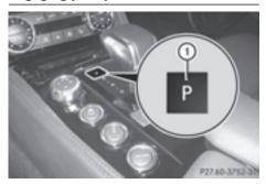
▶ When the vehicle is stationary, press button ①.
