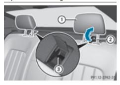
Top Tether anchorage points (3) are installed in the rear compartment behind the outer head restraints.
