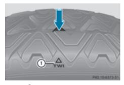
Marking (1) shows where the bar indicator (arrow) for tread wear is integrated into the tire tread.
