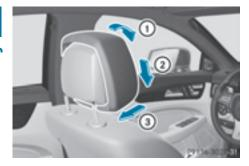
Do not insert your finger between the cushion of the head restraint and the cover. Pay particular attention while resetting the NECK-PRO head restraints.
