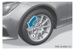
► Using lug wrench ③, loosen the bolts on the wheel you wish to change by about one full turn. Do not unscrew the bolts completely.
