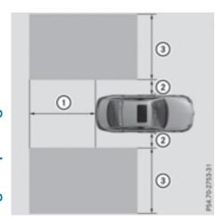
At a distance of approximately 1.6 ft (0.5 m) ② from the vehicle, Blind Spot Assist monitors the area up to 10 ft (3 m) next to ③ and behind ① your vehicle, as shown in the picture.
