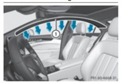
Window curtain air bags ① are integrated into the side of the roof frame and deployed in the area from the A-pillar to the C-pillar.
