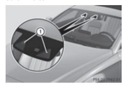
DISTRONIC PLUS with Steering Assist and Stop&Go Pilot aids you in keeping the vehicle in the center of the driving lane by means of moderate steering interventions in a speed range from 0 - 125 mph (0 - 200 km/h).
