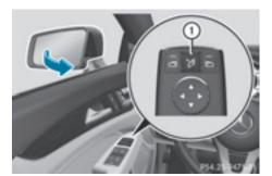
If you have switched on the Auto. Mirror Folding function and you fold in the exterior mirrors by pressing button ①, the exterior mirrors will not fold out automatically ( $\triangleright$  page 101). You can then only fold out the exterior mirrors using button ①.
