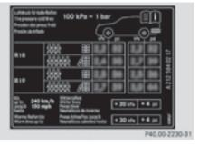
Some tire pressure tables show only the rim diameters instead of the full tire size, e.g. **R18**. Rim diameter is part of the tire size and can be found on the tire sidewall (> page 307).
