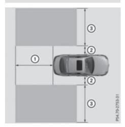
At a distance of approximately 1.6 ft (0.5 m) ② from the vehicle, Active Blind Spot Assist monitors the area up to 10 ft (3 m) next to ③ and behind ① your vehicle, as shown in the picture.
