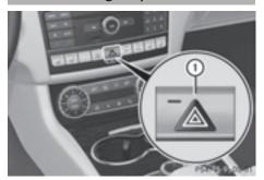
➤ To switch the hazard warning lamps on or off: press button (1).
