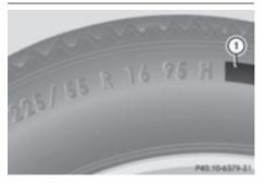
In addition to the load bearing index, load index ① may be imprinted after the letters that identify speed index ⑥ on the sidewall of the tire ( $\triangleright$  page 307).
