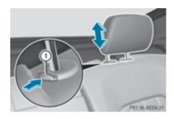
The head restraints can only be removed if the rear seat folds forward.
