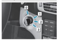
To remove the SmartKey (shift the transmission to position P)
