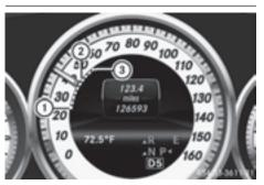
When DISTRONIC PLUS is activated, one or two segments ② in the set speed range light up. If DISTRONIC PLUS detects a vehicle in front, segments ② between speed of the vehicle in front ① and stored speed ③ light up.
