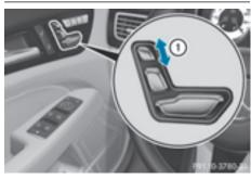
▶ Slide switch for head restraint height adjustment (1) up or down in the direction of the arrow.
