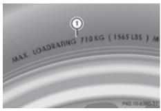
Maximum tire load ① is the maximum permissible weight for which the tire is approved. Do not overload the tires by exceeding the specified load limit. The maximum permissible load can be found on the vehicle's Tire and Loading Information placard on the B-pillar on the driver's side (▷ page 302).
