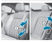
Front side impact air bags (1) and rear side impact air bags (2) deploy next to the outer bolster of the seat backrest.
