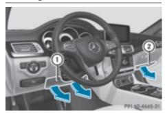
Driver's knee bag ① deploys under the steering column and front-passenger knee bag ② under the glove box. The driver's and front-passenger knee bags are triggered together with the front air bags.
