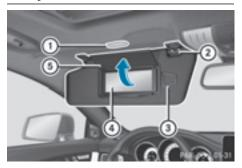
Mirror light ① only functions if the sun visor is clipped into bracket ② and mirror cover ⑤ has been folded up.
