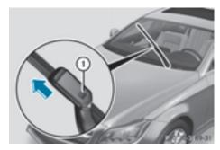
▶ Firmly press release knob (1) and pull the wiper blade upwards from the wiper arm in the direction of the arrow.
