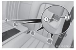
When installing the LATCH-type (ISOFIX) child restraint system, fold protective caps (2) of securing rings (1) inwards.
