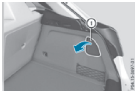
Right-hand side trim panel
