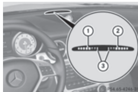
Warning display for the front area
