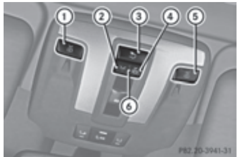
Front overhead control panel
