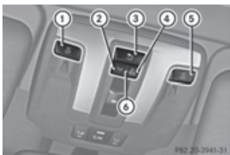
Front overhead control panel
