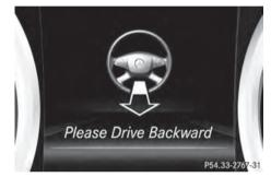
Press the OK button on the multifunction steering wheel to confirm. The multifunction display switches to Parking Guidance.
