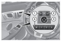
You can position the front-passenger side exterior mirror in such a way that you can see the rear wheel on that side as soon as you engage reverse gear. This setting can be stored using memory button  $\mathbf{M}$  (4).
