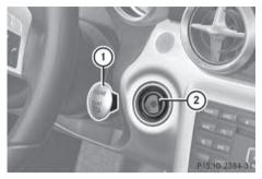
You can remove the Start/Stop button from the ignition lock and start the vehicle as normal using the SmartKey.
