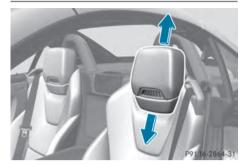
To raise/lower: push the head restraint upwards or pull it down into the desired position.
