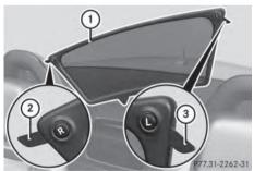
Preparing for installation from the left side of the vehicle (example)
