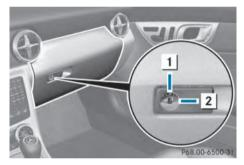
The glove box can be locked and unlocked using the mechanical key.
