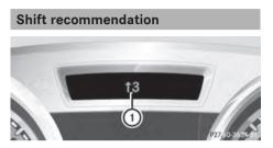
Shift gear according to gearshift recommendation (1) when shown in the multifunction display of the instrument cluster.
