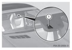
Lane Keeping Assist monitors the area in front of your vehicle with camera (), which is mounted at the top of the windshield. Lane Keeping Assist detects lane markings on the road and warns you before you leave your lane unintentionally.
