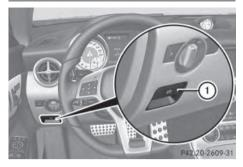
► To engage: push handle ①. When the electric parking brake is engaged, the PARK (USA only) or () (Canada only) red indicator lamp lights up in the instrument cluster.
