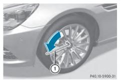
Using lug wrench ①, loosen the bolts on the wheel you wish to change by about one full turn. Do not unscrew the bolts completely. AMG vehicles and vehicles with AMG equipment: to protect the vehicle body, the vehicle has covers next to the jacking points on the outer sills.
