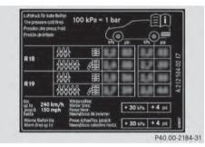
Some tire pressure tables show only the rim diameters instead of the full tire size, e.g. **R18**. The rim diameter is part of the tire size and can be found on the tire sidewall ( $\triangleright$  page 322).
