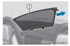
Removing from the left side of the vehicle (example)
