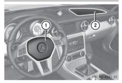
Driver's air bag ① deploys in front of the steering wheel; front-passenger front air bag ② deploys in front of and above the glove box.
