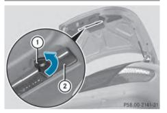
Warning triangle 2 is secured on the inside of the trunk lid.
