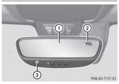
Compass (2) displays the compass direction in which the vehicle is currently traveling: N, NE, E, SE, S, SW, W or NW.
