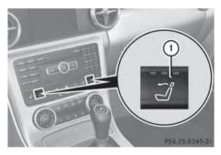
The AIRSCARF function warms the head and neck area of vehicle occupants with warm air. The warm air flows out of the holes in the head restraints.
