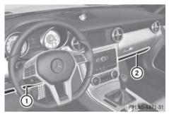
Driver's knee bag ① deploys underneath the steering column and front-passenger knee bag ② underneath the glove box. They deploy together with the front air bags. They are designed to operate together with the front air bags in frontal impacts if certain thresholds are exceeded. The knee bags
