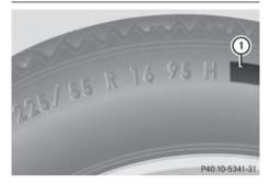
In addition to the load bearing index, load rating (1) may be imprinted after the letters that identify speed rating on the sidewall of the tire ( $\triangleright$  page 322).
