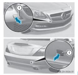
The mountings for the removable towing eyes are located in the bumpers. They are at the front and at the rear, behind the covers.
