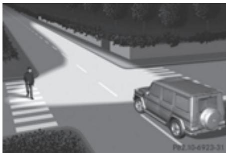
The cornering light function improves the illumination of the road over a wide angle in the direction you are turning, enabling better visibility in tight bends, for example. The cornering light function can only be activated if the low-beam headlamps are switched on and the fog lamps are switched off.
