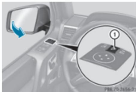
If the battery has been disconnected or completely discharged, the exterior mirrors must be reset. The exterior mirrors will otherwise not fold in when you select the
