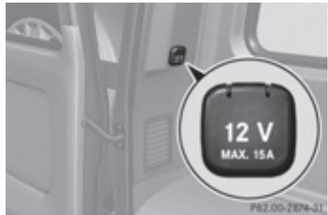
The socket is located in the cargo compartment on the left-hand side, when viewed in the direction of travel, next to the rear door.
