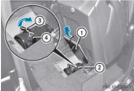
The jack is located under the rear bench seat on the right-hand side when viewed in the direction of travel.
