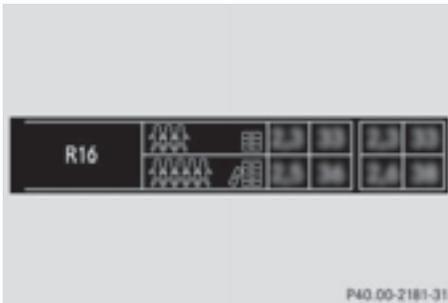
Some tire pressure tables only show the rim diameter instead of the complete tire size, e.g. **R16**. The rim diameter is part of the tire size and can be found on the tire sidewall (▷ page 328).
