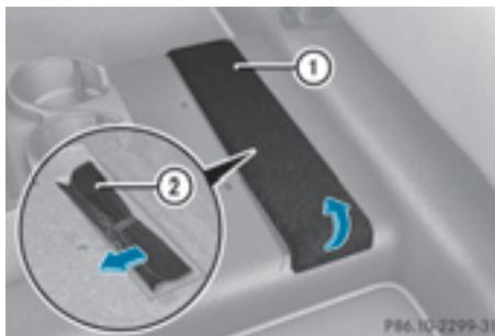
The vehicle tool kit is under the cover in the footwell in front of the rear bench seat.
