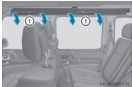
Window curtain air bags ① enhance the level of protection for the head, but not chest or arms, of the vehicle occupants on the side of the vehicle on which the impact occurs.
