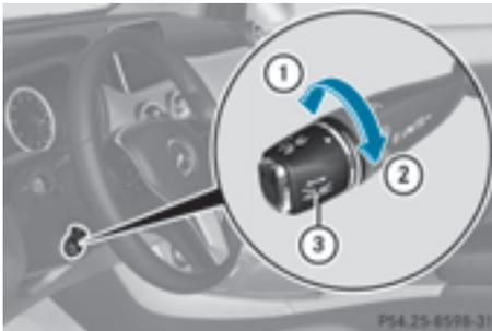
You can set the specified minimum distance for DISTRONIC PLUS by varying the time span between one and two seconds. With this function, you can set the minimum distance that DISTRONIC PLUS keeps to the vehicle in front, dependent on vehicle speed. You can see this distance in the multifunction display (▷ page 213).
