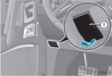
The release lever on the hood is in the footwell on the left-hand side of the vehicle when viewed in the direction of travel.
