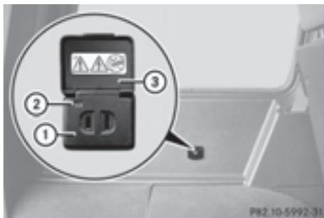
115 V power socket ① provides an AC voltage of 115 V so that small electronic devices can be connected. These devices, such as games consoles, chargers and laptops, should not consume more than a maximum of 150 W altogether.
