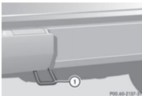
Rear towing eye ① is located under the bumper, on the left-hand side when viewed in the direction of travel.
