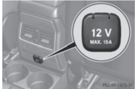
The socket is located on the center console in the rear compartment.
