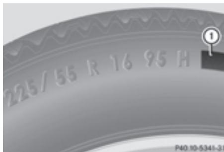
In addition to the load bearing index, load rating **1** may be imprinted after the letters that identify speed rating **6** on the sidewall of the tire (▷ page 328).
