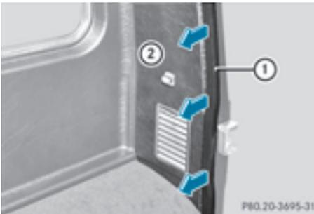
The emergency release is located in the cargo compartment, on the right-hand side when viewed in the direction of travel, behind the rear panel trim.
