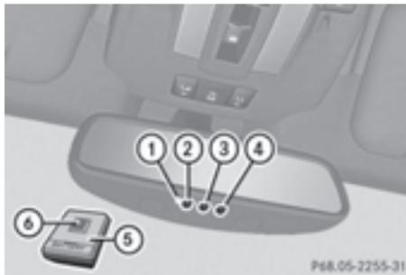
Integrated remote control in the rear-view mirror
