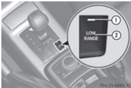
**i** **AMG vehicles:** to shift the transfer case to **LOW RANGE**, deactivate the ECO start/stop function (> page 142).
