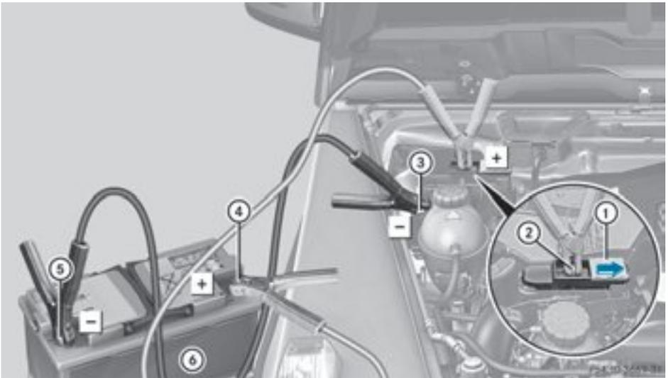
Position number ⑥ identifies the charged battery of the other vehicle or an equivalent jump-starting device.
