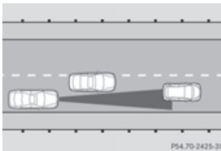
DISTRONIC PLUS may not detect vehicles traveling on a different line. The distance to the vehicle in front will be too short.
