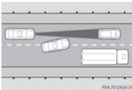
DISTRONIC PLUS has not detected the vehicle cutting in yet. The distance to this vehicle will be too short.
