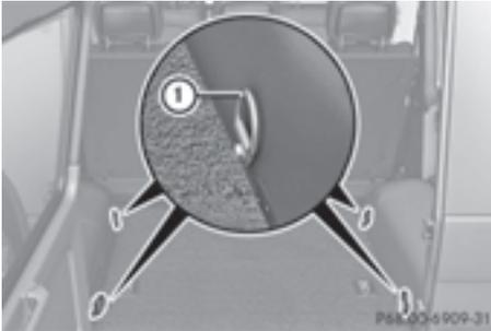
There are four cargo tie down rings (1) in the cargo compartment mounted at the sides.
