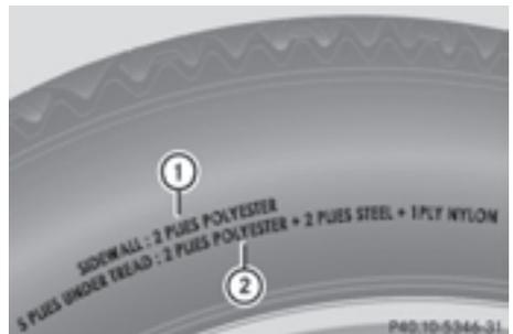
This information describes the type of tire cord and the number of layers in sidewall ① and under tire tread ②.
