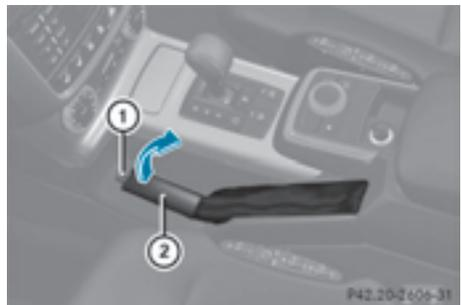
**i** When you apply parking brake ② to brake the vehicle, the brake lamps do not light up.
