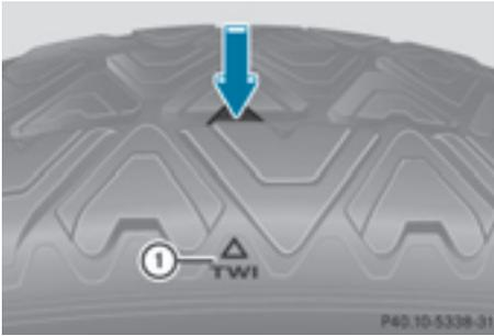
Marking ① shows the tread wear indicator (TWI). The arrow indicates the placement of the tire tread.
