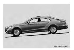
Securing the vehicle on slight downhill gradients
