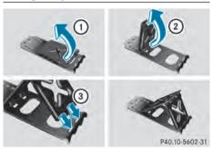
If your vehicle is equipped with a wheel chock, it can be found in the tire-change tool kit (> page 320).
