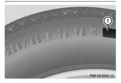
In addition to the load bearing index, load index 1 may be imprinted after the letters that identify speed index 6 on the sidewall of the tire ( $\triangleright$  page 351).
