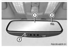
To receive a correct display in rear-view mirror ①, the compass must be calibrated and the magnetic field zone set.
