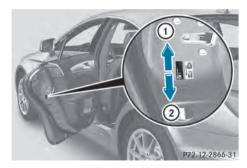
You secure each door individually with the child-proof locks on the rear doors. A door secured with a child-proof lock cannot be opened from inside the vehicle. When the vehicle is unlocked, the door can be opened from the outside.
