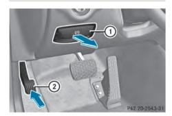
If you brake the vehicle with the parking brake, the brake lamps will not light up.
