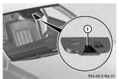
In addition to the illumination provided by the normal headlamps, Night View Assist Plus uses infrared light to illuminate the road. Night View Assist Plus camera ① picks up the infrared light and displays a monochrome image in COMAND. The image displayed in COMAND corresponds to a road lit up by highbeam headlamps. This enables you to see the road's course and any obstacles in good time. If pedestrian recognition is activated, pedestrians recognized by the system are
