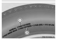
This information describes the type of tire cord and the number of layers in sidewall (1) and under tire tread (2).
