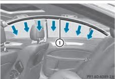
Window curtain air bags ① enhance the level of protection for the head, but not chest or arms, of the vehicle occupants on the side of the vehicle on which the impact occurs.
