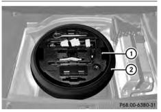
The emergency spare wheel can be found in the stowage well under the trunk floor.
