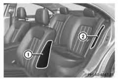
Front side impact air bags ① and rear side impact air bags ② deploy next to the outer seat cushions.
