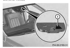
Active Lane Keeping Assist monitors the area in front of your vehicle by means of camera (1) at the top of the windshield. Active Lane Keeping Assist detects lane markings on the road and warns you before you leave your lane unintentionally. If you do not react to the warning, a lane-correcting application of the brakes can bring the vehicle back into the original lane.
