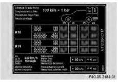
Some tire pressure tables show only the rim diameters instead of the full tire size, e.g. **R18**. The rim diameter is part of the tire size and can be found on the tire sidewall (⊳ page 351).
