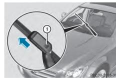
► Firmly press release knob ① and pull the wiper blade upwards from the wiper arm in the direction of the arrow.
