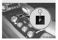
► When the vehicle is stationary, press P button (1).
