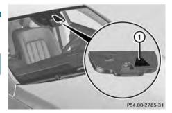
Lane Keeping Assist monitors the area in front of your vehicle with camera ①, which is mounted at the top of the windshield. Lane Keeping Assist detects lane markings on the road and warns you before you leave your lane unintentionally.
