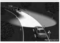
The active light function is a system that moves the headlamps according to the steering movements of the front wheels. In this way, relevant areas remain illuminated while driving. This allows you to identify pedestrians, cyclists and animals.
