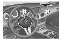
Driver's air bag ① deploys in front of the steering wheel; front-passenger front air bag ② deploys in front of and above the glove box.
