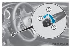
You can set the specified minimum distance for DISTRONIC PLUS by varying the time span between one and two seconds. With this function, you can set the minimum distance that DISTRONIC PLUS keeps to the vehicle in front, dependent on vehicle speed. You can see this distance in the multifunction display (> page 184).
