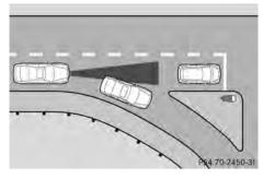
DISTRONIC PLUS does not brake for obstacles or stationary vehicles. If, for
