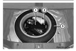
The emergency spare wheel can be found in the stowage well under the trunk floor.
