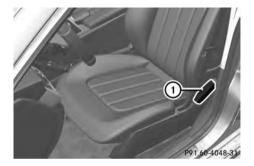
Pelvis air bags ① enhance the level of protection of the vehicle occupants on the side of the vehicle on which the impact occurs.
