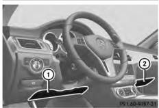
Driver's knee bag (1) deploys underneath the steering column and front-passenger knee bag (2) underneath the glove box. They deploy together with the front air bags. They are designed to operate together with the front air bags in frontal impacts if certain thresholds are exceeded. The knee bags operate at best in conjunction with correctly positioned and fastened seat belts.
