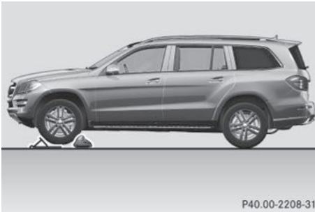
Securing the vehicle on level ground
