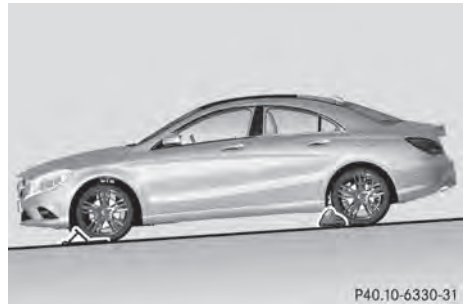
Securing the vehicle on slight downhill gradients
