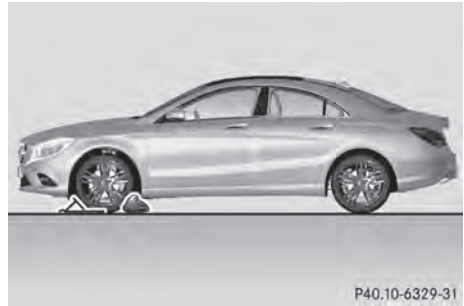
Securing the vehicle on level ground
