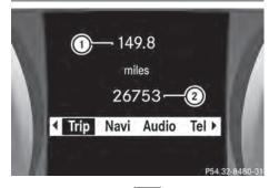
Press and hold the <u>steering</u> button on the steering wheel until the Trip (1) menu with trip odometer 1 and odometer 2 is shown. (2)
