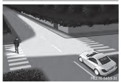
The cornering light function improves the illumination of the road over a wide angle in the direction you are turning, enabling better visibility in tight bends, for example. The cornering light function can only be activated when the low-beam headlamps are switched on.
