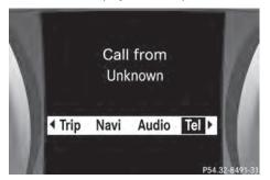
Press the button on the steering wheel to accept an incoming call.
