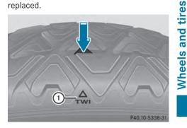
Bar marking ① for tread wear is integrated into the tire tread.
