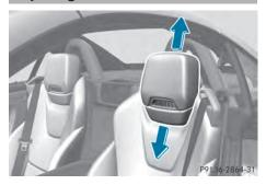
To raise/lower: push the head restraint upwards or pull it down into the desired position.
