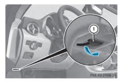
Pull release lever (1) for the hood. The hood is released.
