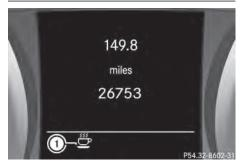
► Activate ATTENTION ASSIST using the onboard computer (▷ page 191). Symbol ① appears in the multifunction display.
