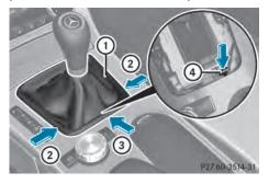
Do not use any sharp-edged objects to remove the selector lever gaiter from the center console. This could damage the selector lever gaiter.
