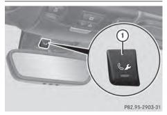
Press and hold Roadside Assistance button ① for more than two seconds. This initiates a call to the Mercedes-Benz Customer Assistance Center. The indicator lamp in Roadside Assistance button ① flashes while the call is active. The Connecting Call message appears in the multifunction display. The audio output is muted.
