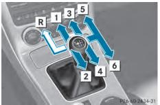
Gear lever R Reverse gear 1 to 6 Forward gears multifunction display of the instrument cluster.
