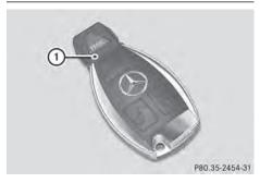
Press the g or g button. The battery is working properly if battery check lamp (1) lights up briefly
