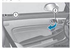
Pull door handle ②. If the door is locked, locking knob ① pops up The door is uplealed and eap handle.
