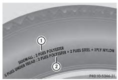
**1** Tire data is vehicle-specific and may deviate from the data in the example.
