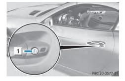
Turn the mechanical key counter-clockwise to position 1.
