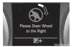
▶ While the vehicle is stationary, turn the steering wheel in the specified direction
