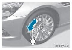
Using lug wrench (1), loosen the bolts on the wheel you wish to change by about one full turn. Do not unscrew the bolts completely.
