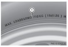
Maximum load rating ① is the maximum permissible weight for which the tire is approved.
