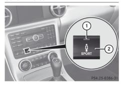
The adjustable damping system adapts to the current driving conditions. The adjustment depends on whether you have selected sport or comfort mode. Your selection remains stored even if you remove the SmartKey from the ignition lock.
