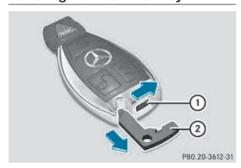
▶ Push release catch (1) in the direction of the arrow and at the same time, remove mechanical key (2) from the SmartKey.
