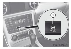
▶ To deactivate: press button (1) until the ESP® OFF warning lamp lights up in the instrument cluster.
