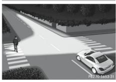
The cornering light function improves the illumination of the road over a wide angle in the direction you are turning, enabling better visibility in tight bends, for example. The cornering light function can only be activated
