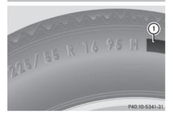
In addition to the load bearing index, load rating 1 may be imprinted after the letters that identify speed rating on the sidewall of the tire ( $\triangleright$  page 323).
