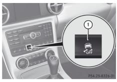
► To switch off: press button (1). The [基] ESP® OFF warning lamp in the instrument cluster lights up.
