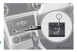
The AIRSCARF function warms the head and neck area of vehicle occupants with warm air. The warm air flows out of the holes in the head restraints.
