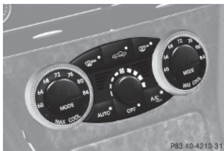
Automatic climate control panel with MAX COOL activated
