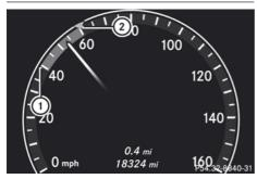
When you switch on DISTRONIC PLUS, triangle (2) shows the stored speed.
