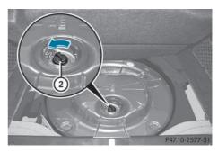
► Turn DEF filler cap ② counter-clockwise and open it. Filler cap ② is secured with a plastic strap.
