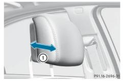
▶ Pull or push the bottom of NECK-PRO head restraint (1).
