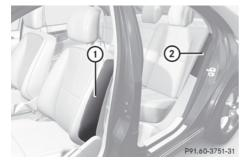
Front side impact air bags (1) and rear side impact air bags (2) deploy next to the outer seat cushions.
