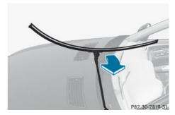
Remove the wiper blade from the retaining pin on the wiper arm in the direction of the arrow.
