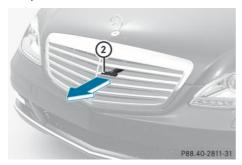
▶ Pull hood catch handle ② outwards from the radiator grill as far as it will go and lift the hood from underneath by the radiator grill.
