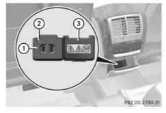
115 V socket (1) provides an alternating voltage of 115 V, so that small electronic devices can be connected. These devices,
