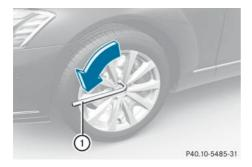
▶ Using lug wrench (1), loosen the bolts on the wheel you wish to change by about one full turn. Do not unscrew the bolts completely.
