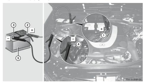
Position number (5) identifies the charged battery of the other vehicle or an equivalent jump-starting device.
