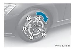
➤ Tighten the wheel bolts evenly in a crosswise pattern in the sequence indicated (① to ⑤). The tightening torque must be 110 lb-ft (150 Nm).
