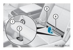
Installation instructions (1) indicate the installation location of securing rings (2).
