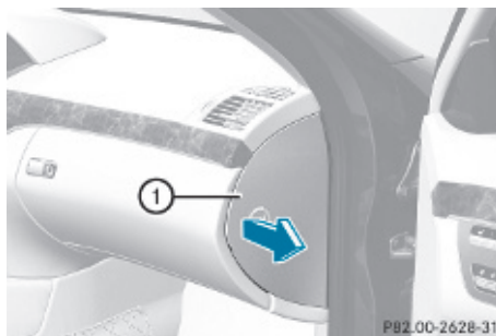
Fuse box on passenger side
