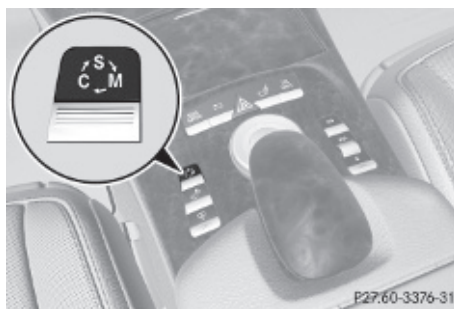
Program mode selector switch on AMG vehicles
