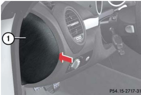
① Fuse box cover
