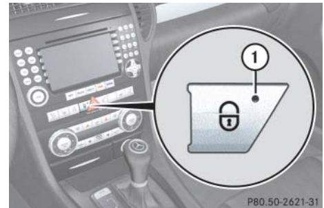
① Alarm system indicator lamp
