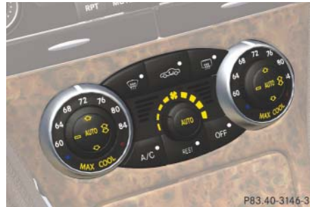
Automatic climate control panel with MAXCOOL activated
