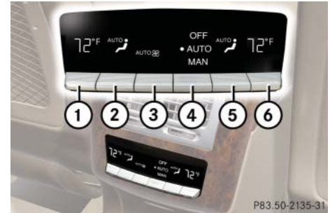
Automatic climate control panel, rear
