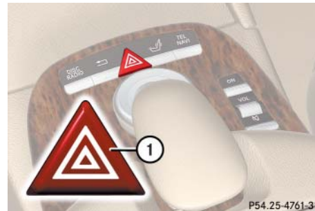
① Hazard warning flasher switch
