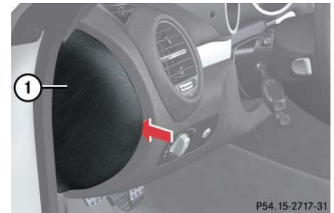
① Fuse box cover
