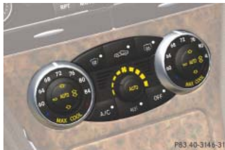
Automatic climate control panel with MAXCOOL activated
