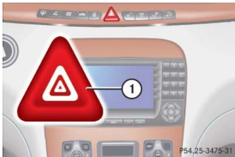
① Hazard warning flasher switch
