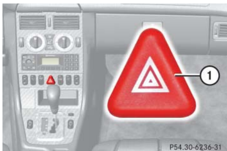
① Hazard warning flasher switch
