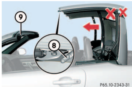
8 Pins for the retractable hardtop locking mechanism
