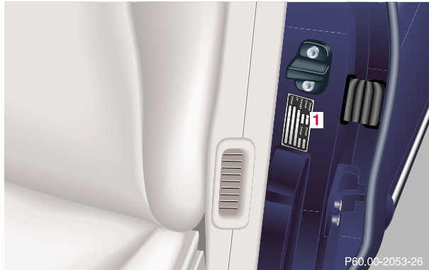
1 Certification label (below driver's door lock latch)
