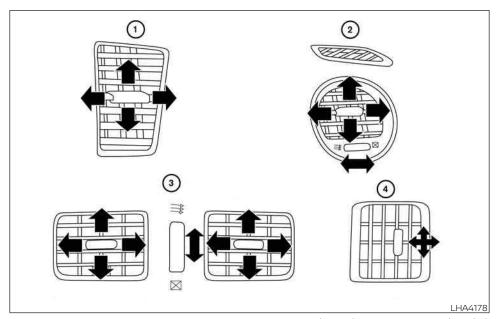
Adjust air flow direction for the center vents 1), driver's and passenger's side vents 2), rear center console vents (3), and rear passenger compartment vents (4) by moving the vent slide and/or vent assemblies.
