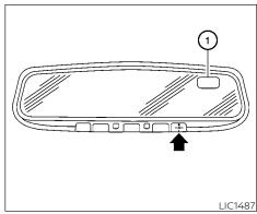
If the display reads "C", calibrate the compass by driving the vehicle in three complete circles at less than 5 mph (8 km/h).
