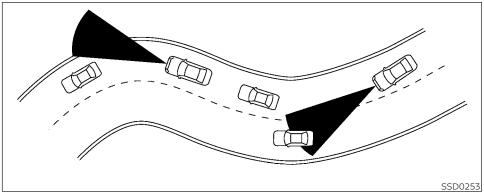
When driving on some roads such as winding, hilly, curved, narrow roads, or roads which are under construction, the sensor may detect vehicles in a different lane, or may temporarily not detect a vehicle traveling ahead. This may cause the system to work inappropriately.
