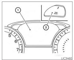
Odometer/Twin trip odometer
