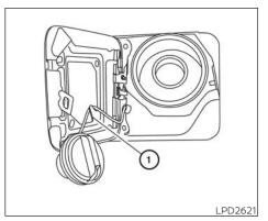
To remove the fuel-filler cap:
