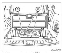
3. Remove the tool kit © by releasing the Velcro straps (D).
