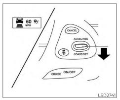
**To set cruising speed,** accelerate your vehicle to the desired speed, push the COAST/SET switch and release it. The ICC system set indicator (green), vehicle ahead detection indicator, set distance indicator and set vehicle speed indicator **®** will come on. Take your foot off the accelerator pedal. Your vehicle will maintain the set speed.
