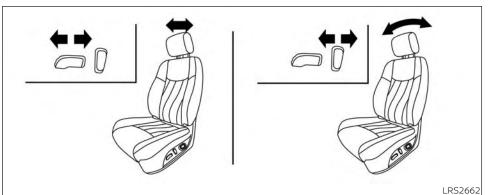
FRONT POWER SEAT ADJUSTMENT (if so equipped)
