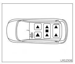
The illustration shows the seating positions with head equipped restraints/headrests.
