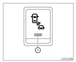
The warning systems switch is used to turn on and off the Blind Spot Warning (BSW) system that is activated using the settings menu on the vehicle information displav.
