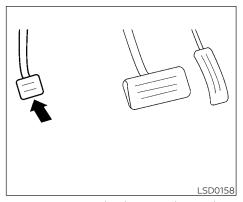
To engage: Firmly depress the parking brake
