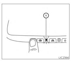
2. Using both hands, simultaneously press and hold the desired HomeLink® button and hand-held transmitter button DO NOT release until the HomeLink® indicator light (1) flashes slowly and then rapidly. When the indicator light flashes rapidly, both buttons may be released. (The rapid flashing indicates successful programming.)
