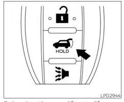
Releasing the rear liftgate (if so equipped)
