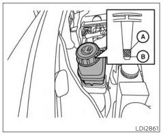
Check the fluid level in the reservoir
