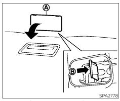
Power liftgate release (if so equipped)
