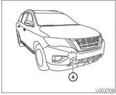
The AEB system uses a radar sensor (A) located behind the lower grille of the front bumper to measure the distance to the vehicle ahead in the same lane.
