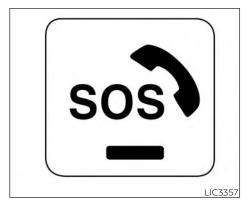
The E-call (SOS) button is used in combination with a NissanConnect® Services subscription to call for assistance in case of an emergency.
