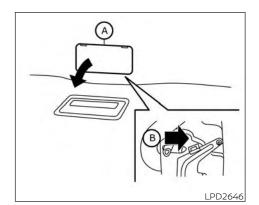
Manual liftgate release (if so equipped)
