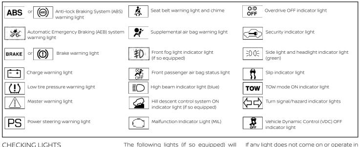
With all doors closed, apply the parking brake, fasten the seat belts and place the ignition switch in the ON position without starting the engine. The following lights (if so equipped) will come on:
