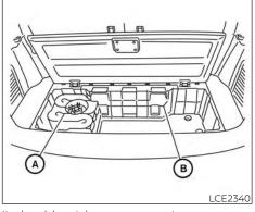
It should not be necessary to remove or dislocate the Bose subwoofer (if so equipped) (A) when removing the jack and tool kit cover (B).
