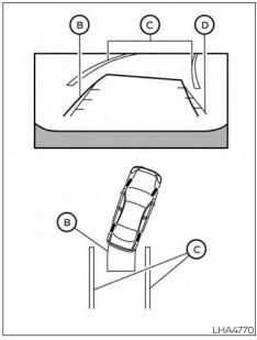
3. Slowly back up the vehicle adjusting the steering wheel so that the predicted course lines (B) enter the parking space (C).
