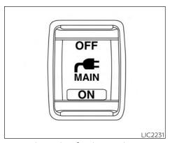
To use the outlets for devices that require 120v power, place the ignition in the ON position and push the power inverter switch.
