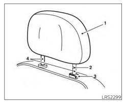
NON-ADJUSTABLE HEAD RESTRAINT/HEADREST COMPONENTS
