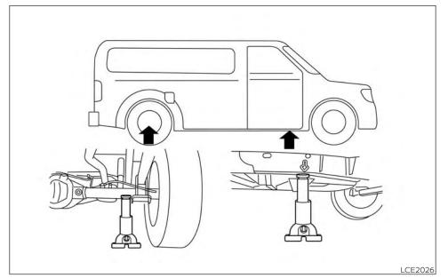
2. Place the jack directly under the jack-up point so the top of the jack contacts the vehicle at the jack-up point. The jack-up points are indicated by stamped arrows on the side of the frame or the rear.
