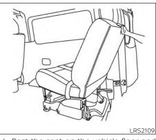
4. Rest the seat on the vehicle floor and with two people, remove the seat from the vehicle. Store the seat in a safe location.
