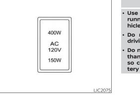
To use the outlets for devices that require 120v power, place the ignition switch in the ON position and push the power inverter switch.
