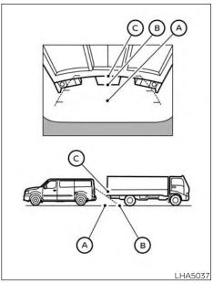
object when backing up to the position (A) if the object projects over the actual backing up course.
