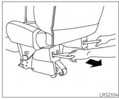
2. Stand directly behind the seat and pull up and rearward on the straps to disengage the seat.
