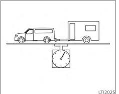
The GCWR equals the combined weight of the towing vehicle (including passengers and cargo) plus the total trailer load. Towing loads greater than these or using improper towing equipment could adversely affect vehicle handling, braking and performance
