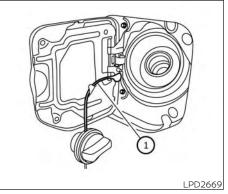
To remove the fuel-filler cap:
