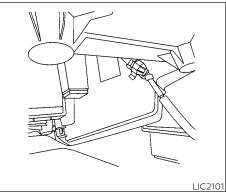
6. The harness cap (if so equipped) is taped to the harness underneath the inside of the center console. Remove the tape to remove the cap.
