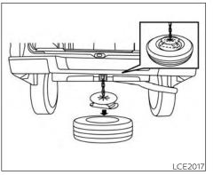
10. To reinstall the wheel, insert the tire chain through the wheel. Be sure the rubber spacer is centered on the wheel before lifting. Use the assembled jack rod and slowly rotate the winch clockwise to raise the wheel to the vehicle.
