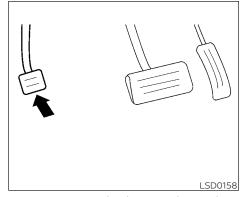
**To engage:** Firmly depress the parking brake.
