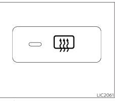
To defrost the rear window glass, place the ignition switch in the ON position and push the rear window defroster switch on. The rear window defroster indicator light comes on. Push the switch again to turn the defroster off.
