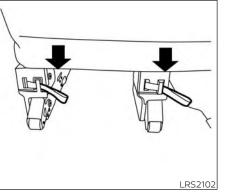
1. Remove the pull strap from the stowed position.
