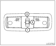
The interior lights have a three-position switch and operate regardless of ignition switch position.
