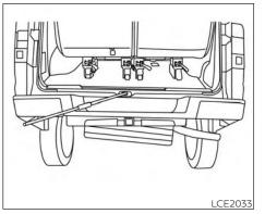
6. Assemble the extension and the J-shaped end tool together before inserting them into the oval-shaped opening above the middle of the rear step bumper. Pass the J-shaped end of the jack rod through the opening and direct it toward the spare tire winch, located directly above the spare tire.
