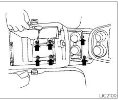
4. Remove the four bolts located inside the console and two in the front storage tray.
