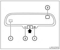
The indicator light 2 will illuminate when the automatic anti-glare feature is operating.
