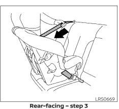
3. Pull the shoulder belt until the belt is fully extended. At this time, the seat belt retractor is in the ALR mode (child restraint mode). It reverts to the ELR mode when the seat belt is fully retracted.
