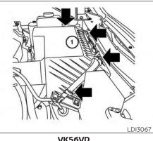
The air cleaner filter should not be cleaned and reused. Replace it according to the maintenance log shown in the "Maintenance and schedules" section of this manual.
