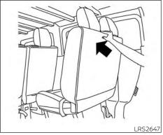
3. Push up and forward to remove the seats from the wells.
