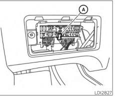
3. Remove the fuse with the fuse puller  $(\underline{A})$ .
