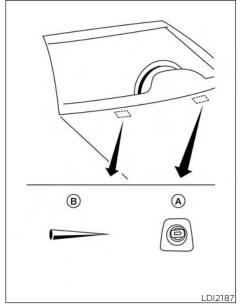
Be careful not to let anything get into the washer nozzle (A). This may cause clogging or improper windshield washer operation. If something gets into the nozzle, remove it with a needle or small pin (B).
