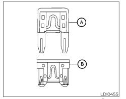
Two types of fuses are used. Type (A) and Type (B) (if so equipped) are used in the fuse boxes in the engine compartment. Type (B) cannot be used to replace Type (A) in the underhood fuse boxes.
