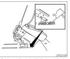
5. Line up the seat with the mounting locations. Tilt the seat slightly forward so the front hooks engage into the front mounting locations.
