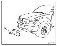
INSTALLING FRONT LICENSE PLATE WITH GROMMETS
