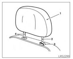
NON-ADJUSTABLE HEAD RESTRAINT/HEADREST **COMPONENTS**
