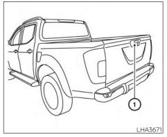
To display the rear view, the Rear View Monitor system uses a camera located next to the tailgate handle (1).
