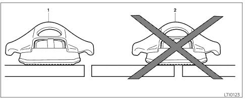
1 correct installation, 2 incorrect installation
