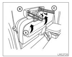
1. To access the jump seat extension (passenger's side only) (a) on the jump seat, pull up (b) on the extension to unfold it to the open position. Then unfold the two support legs (c) and lower the jump seat to the full open seating position.
