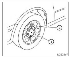
Removing bolt-on wheel caps (if so equipped)
